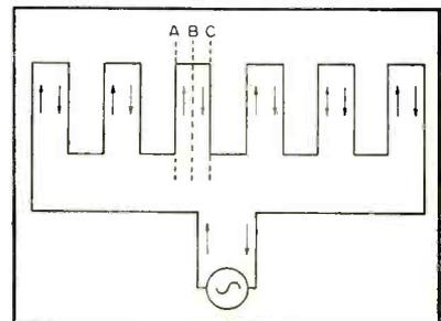
**FIG. 2—Adjacent conductors are 180 deg out of phase causing null point to occur at B**
