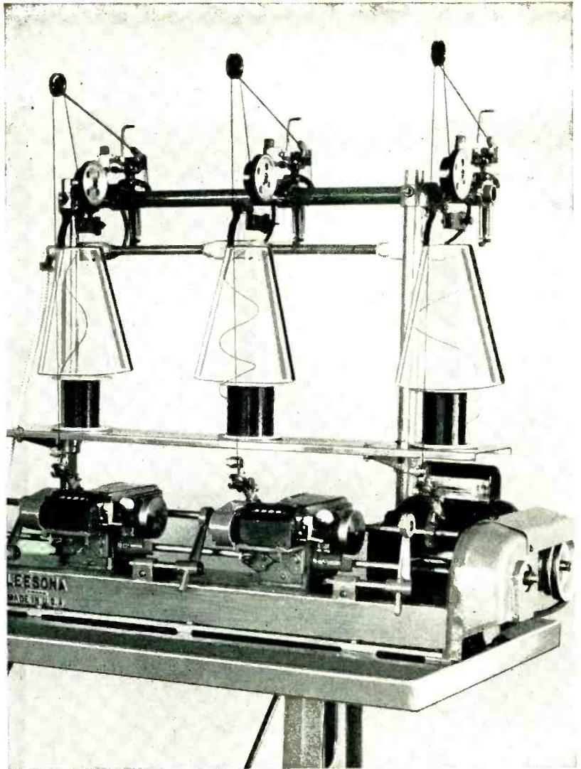
**UNIVERSAL NO. 102 HI-SPEED COIL WINDER** specifically designed for spool-wound coils. Has these desirable characteristics: instant starting over-end tension . . . will accommodate wire size from No. 24 to No. 42 (B&S) . . . can wind two coils per head simultaneously . . . winds up to 4700 rpm, but can be operated at 650 rpm when required.
