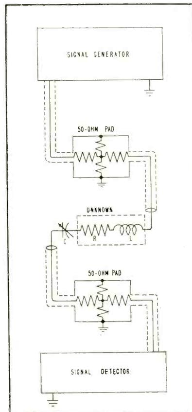
FIG. 1—Insertion-loss measuring circuit used when resistance of the unknown impedance is large compared to the 50-ohm attenuation pads
