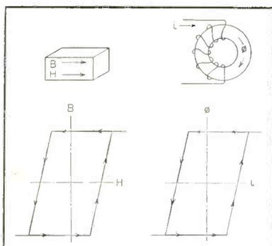
FIG. 1—Characteristic plots for grain-oriented nickel-iron used in magnetic amplifier cores
