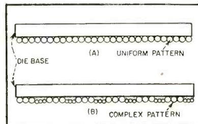
FIG. 6—Uniform (A) or complex (B) pattern depends on die base
