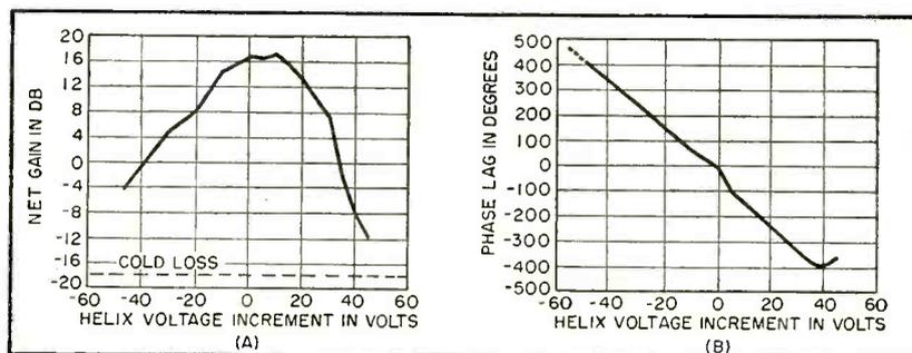
FIG. 3—Phase and gain versus helix voltage for oscillator using tube 135 wavelengths long
