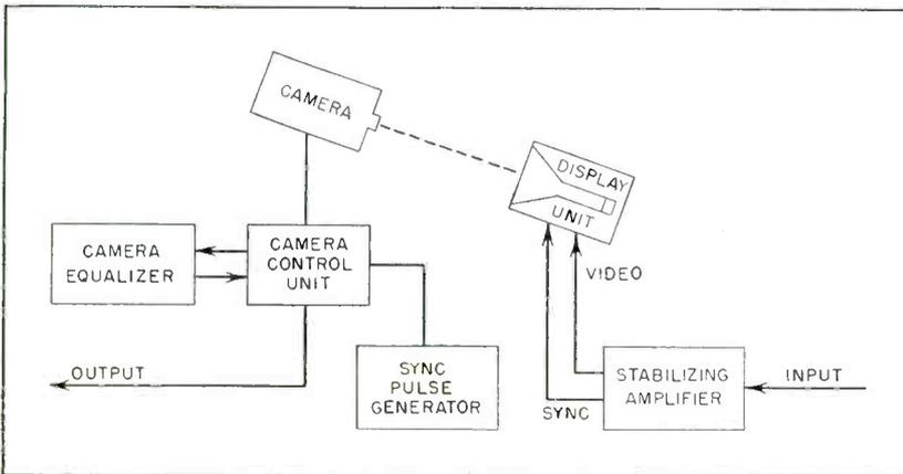
FIG. 1—Scanning-standards converter includes high-quality receiver that presents picture to be converted on long-persistence cathode-ray tube. Resulting optical image is scanned by image-orthicon-type camera operated according to desired scanning standard
