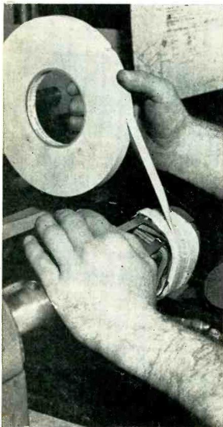
**ANCHORING** sheet leads on this PECO transformer coil requires a strong but not bulky tape. The job is done to order with "Scotch" Electrical Tape No. 45. Sheet leads can be punched, then wired directly to the transformer. No terminal bond is needed.
