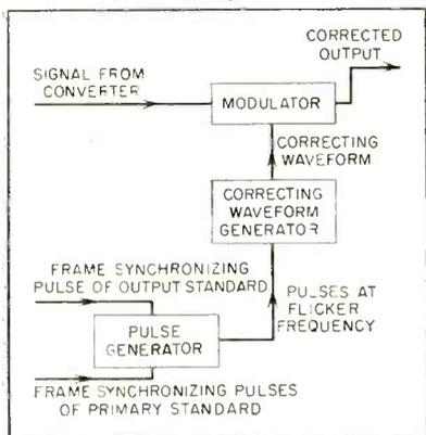
FIG. 5—Suggested method for obtaining flicker-free output when converting from U. S. scanning standards to British
