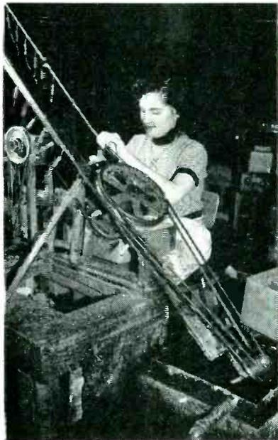
Leather-belt conveyor arrangement for dipping paper capacitors into beeswax in heated tank at lower right
