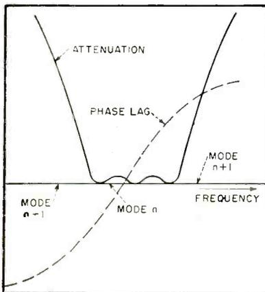
FIG. 2—Phase and attenuation versus frequency for a typical bandpass filter
