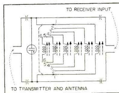
FIG. 2—Antenna duplexer circuit
