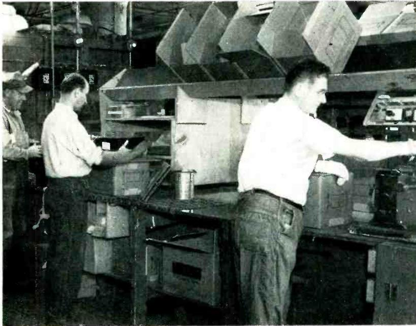
Final packing bench for radio sets. Conveyor line is within easy reach of operator at right, who unloads empty cartons and loads full cartons after sealing them
