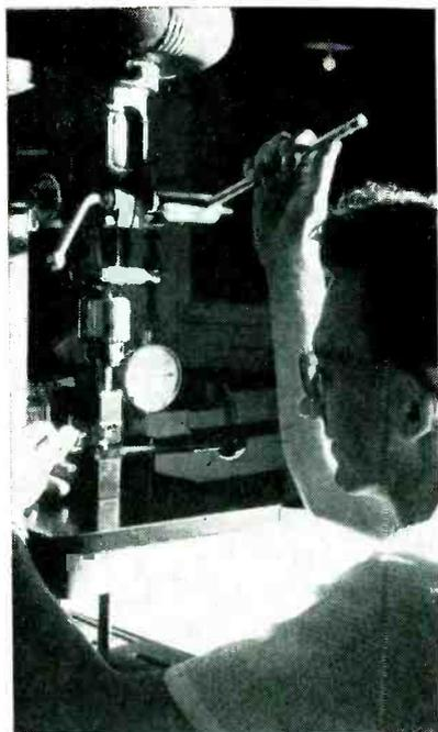
Reducing thickness of moving contact, after removing armature temporarily from relay, by applying pressure with spinning tool while watching resulting change in thickness on dial indicator
