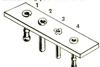
Multi-swaged terminals may be assembled by the following methods: 1. flared; 2. rolled; 3. slitted; or 4. spun. Courtesy The Bead Chain Manufacturing Co., Bridgeport, Conn. (336)
