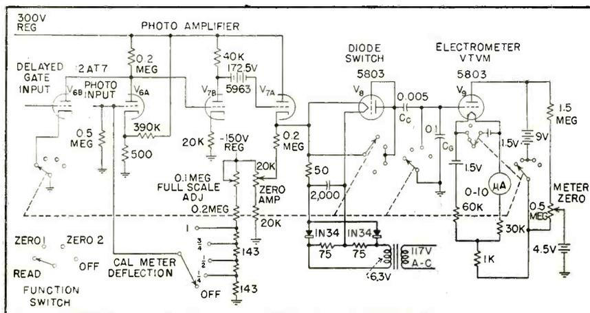
FIG. 3—Gated photo amplifier and electrometer vacuum-tube voltmeter circuits
