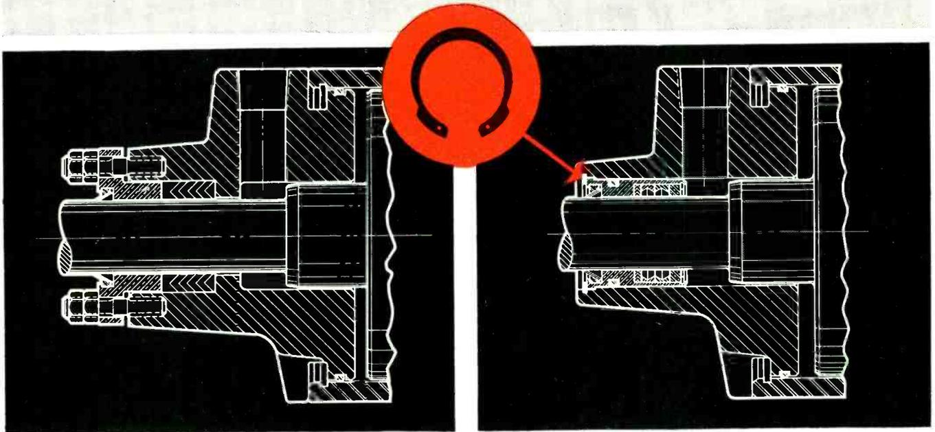
**OLD STYLE** stuffing box required skilled worker to install packing rings one at a time, then adjust packing glands by trial and error. Disassembly was equally difficult, time-consuming and costly.
