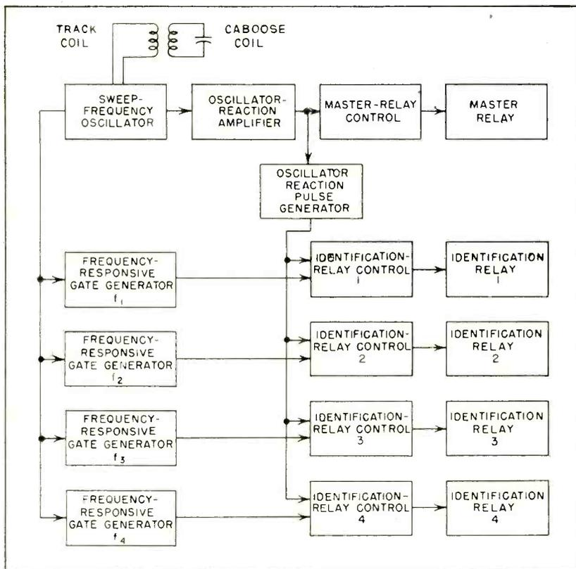
FIG. 4—Electronic train watcher identifies trains passing unattended junction. Train is tagged by tuned circuit suspended below caboose
