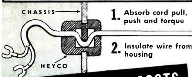
1. Absorb cord pull, push and torque
