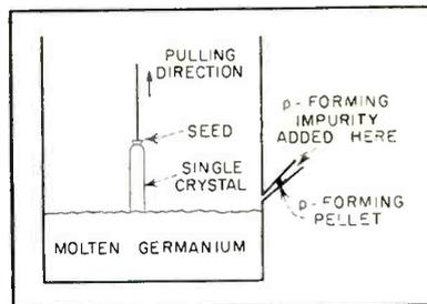
FIG. 5—Sketch indicates technique for preparing grown-junction transistors. The *p*-forming pellet melts and spreads through molten germanium
