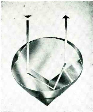
FIG. 1—Prism returns light to its source
