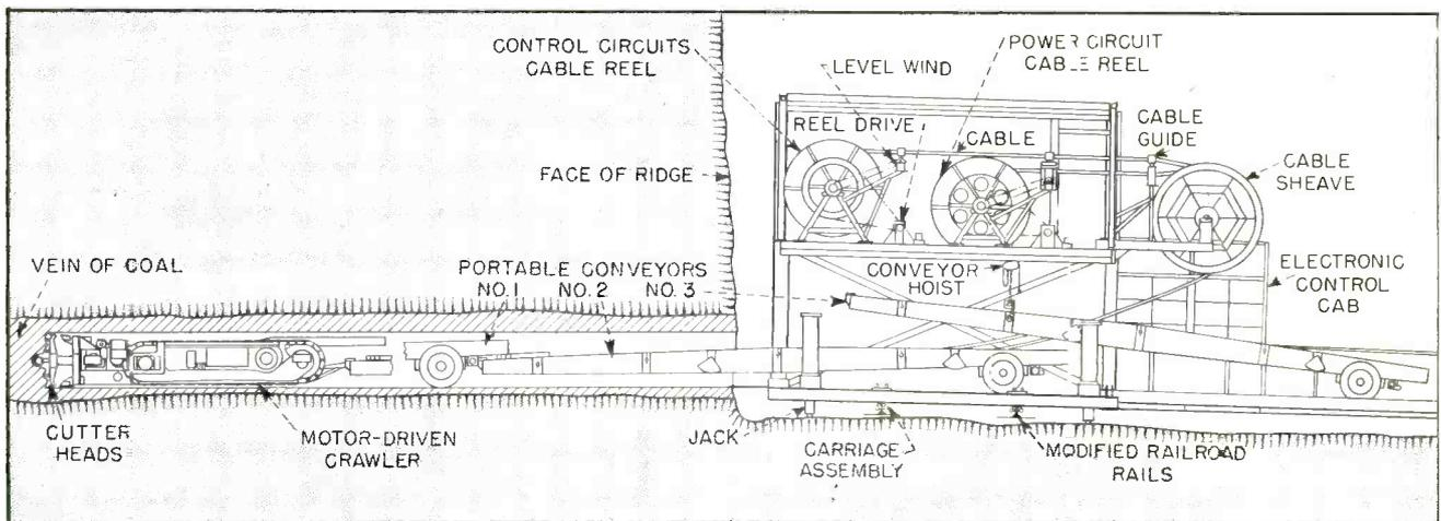
FIG. 1—Side view of new mining machine, which runs on cross rails paralleling face of hill when moving to new position for start of next tunnel. Crawler powered by electric motors supports rotating cutters that break up coal for conveyor feed out of tunnel to waiting trucks. Thirty-foot conveyor sections, added or removed as needed, are towed by crawler as it advances into vein of coal
