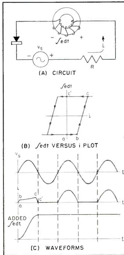
FIG. 3—Crystal diode in simple series circuit. Current on positive half-cycle is determined by  $v_s$  and  $R$
