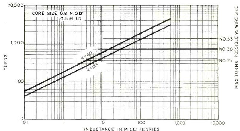
FIG. 3—Master design chart for toroids with 0.8-in. (O. D.) cores
