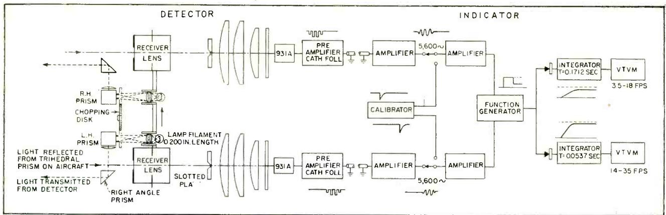
FIG. 2—Block diagram of optical and electronic system of rate-of-descent indicator
