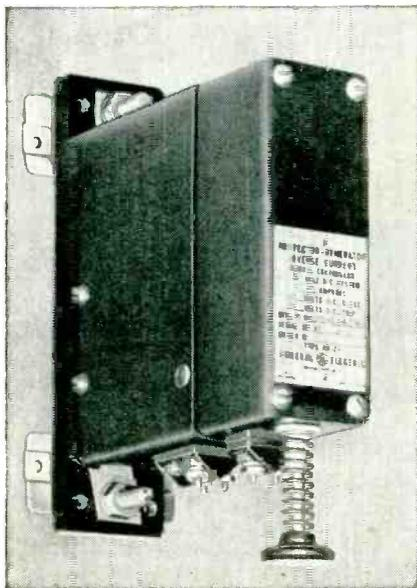
**Circuit Breakers**—Here, a Carboloy magnet assembly simplifies trip element. It eliminates a coil and polarizing connection . . . makes possible reverse-current tripping independent of system voltage. Breaker weighs less, costs less to build.
