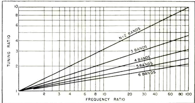
FIG. 1—Chart determines design factors for continuous-coverage tuners having up to six bands
