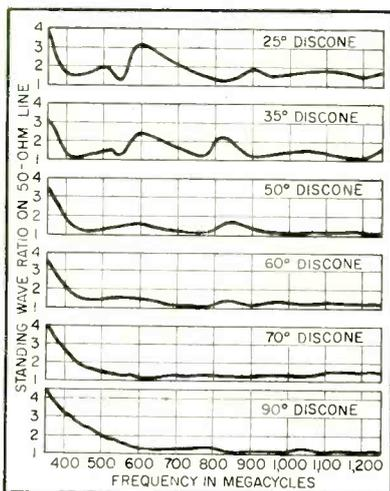
FIG. 4—Standing-wave ratio versus frequency for several discone angles
