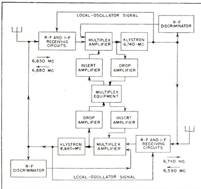
FIG. 2—Microwave repeater used on Santa Fe has single klystron for receiver local oscillator and transmitter
