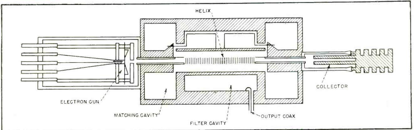
One of the traveling-wave tubes tested in oscillator service. Cutaway shows arrangement of an oscillator circuit
