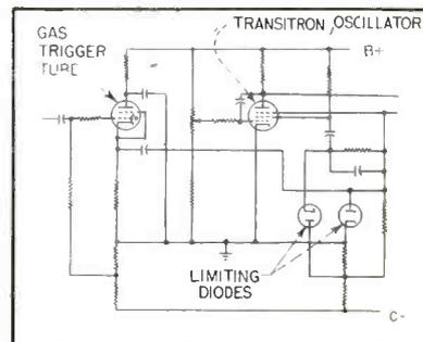
FIG. 2—Transatron oscillator sweep generator
