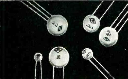
**Ceramic Disc Hi-Kap Capacitors** hold thickness to a minimum . . . have very high capacity in extremely small size. Use in h.f. circuits for bypass and coupling. Ceramic body assures low inductance. Other characteristics—humidity resistance, power factor, etc. — similar to BC Tubulars, Bulletin No. 42-4R.
