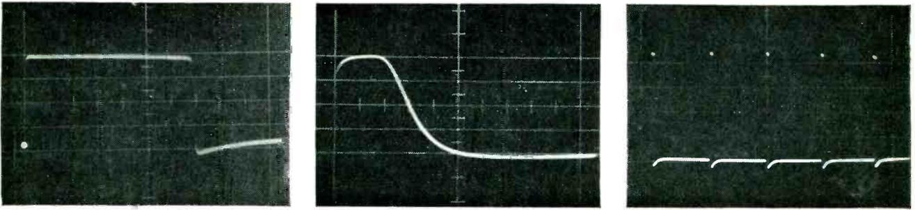
Oscillograms show typical pulses produced by inexpensive pulse circuit. Left to right are pulses of 500  $\mu$ sec at 600 cps, 0.3  $\mu$ sec at 50 kc and a series of 1- $\mu$ sec pulses at 25 kc
