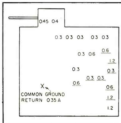
FIG. 3—Drawing shows positions of tubes and filament current of each
