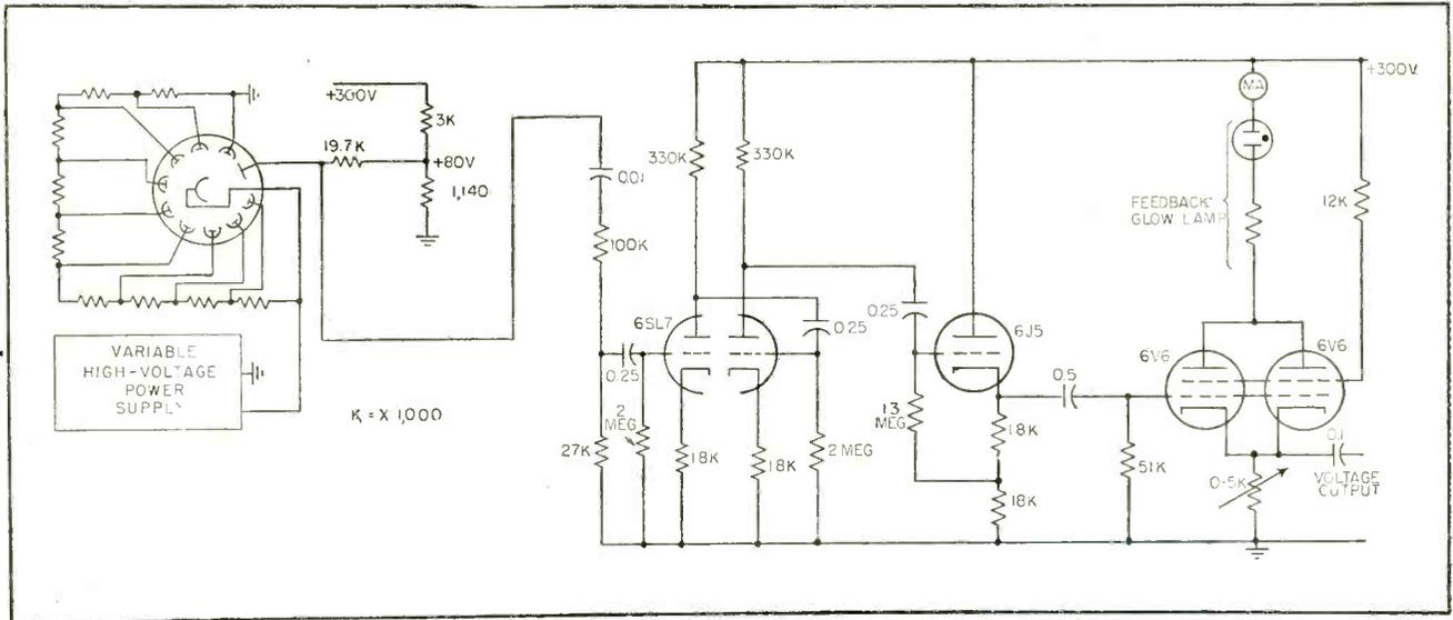
FIG. 2—Multiplier phototube, left, and current amplifier used to invert phase and control glow lamp
