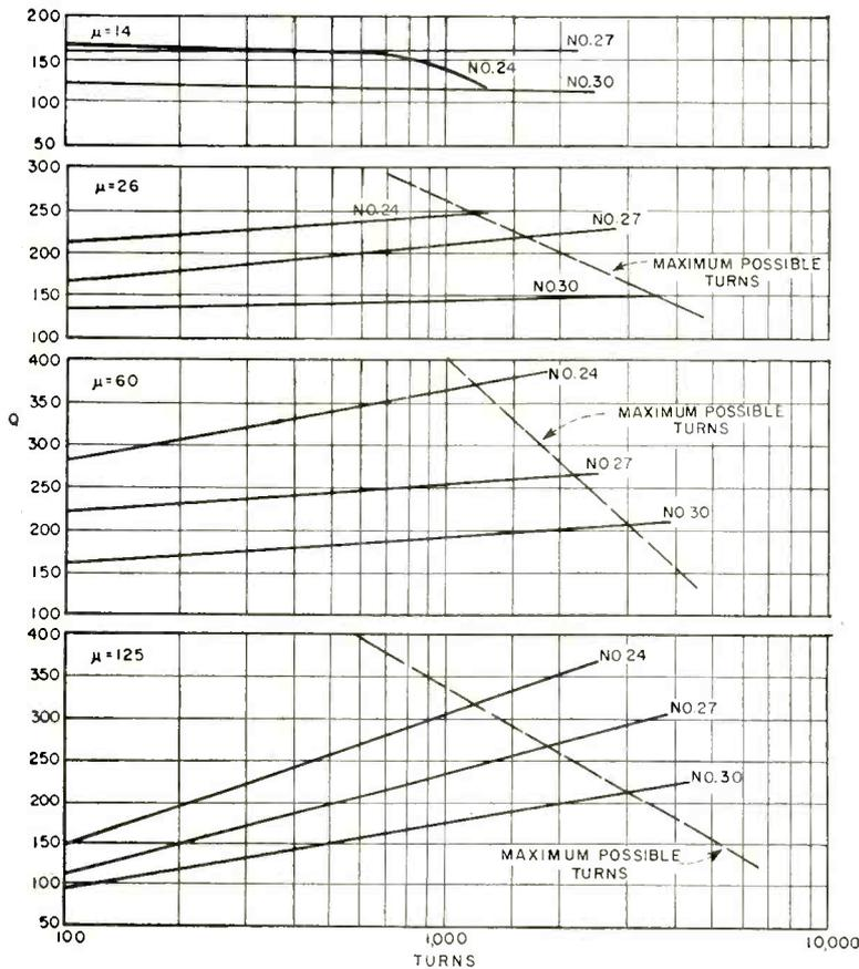
FIG. 4—Auxiliary design chart for toroids using 1.84-in. cores
