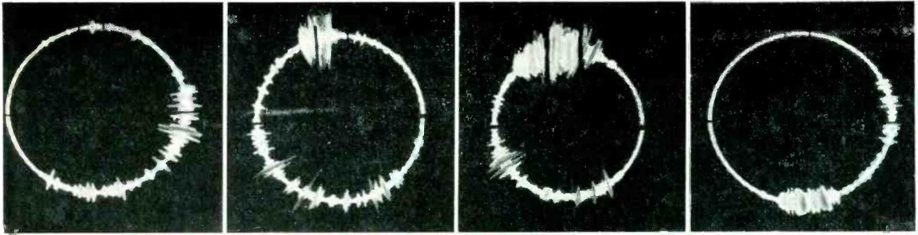
Normal cutting, just hitting draw slate at top or 12 o'clock and going through bone coal strata at about 3:30 o'clock
