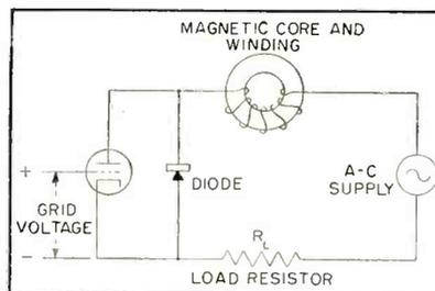
FIG. 7—Vacuum-tube equivalent of magnetic amplifier circuit having grounded-emitter transistor shunted by diode
