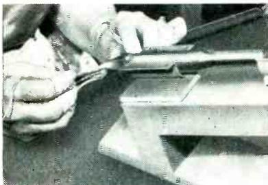
Method of using soldering iron in holder for fastening ferrules to end of shielding braid on cable
