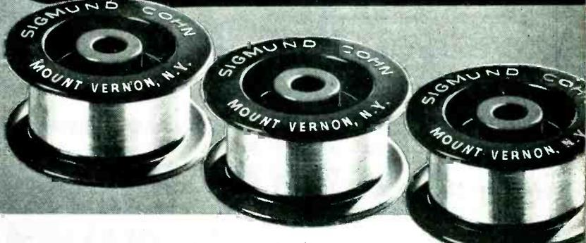
● To meet the growing demand from producers of light-weight, high-frequency Galvanometer movements, we have expanded our facilities designed to process Wire of 2S Aluminum . . . This wire can be supplied in diameters ranging from approximately .001 inch through .005 inch . . . Anodized with exceptionally thin and flexible dielectric coating.
