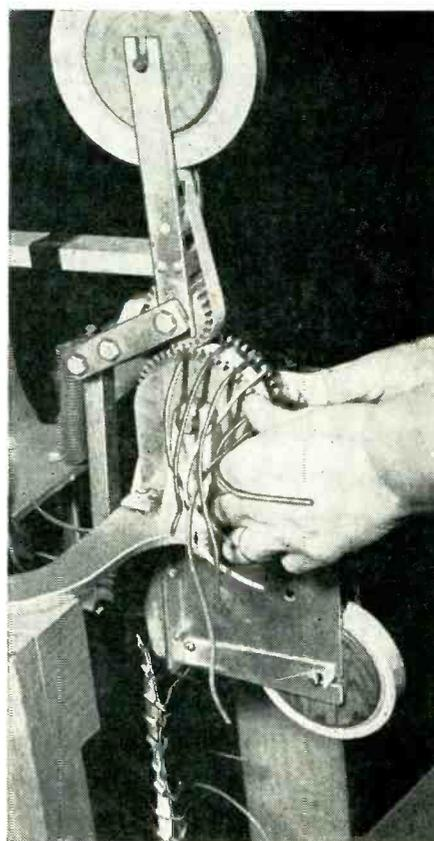
**SADDLING** terminal lead-outs for PECO coils is correctly done with "Scotch" Electrical Tape No. 38. Thermosetting adhesive is heat-cured to form a permanent bond, highly resistant to solvents. Caliper: 10 mils. Dielectric strength: 1500 volts. Treated paper backing.
