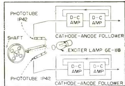
FIG. 1—Shaft position digitizer using serrated drum and phototubes to measure shaft rotation
