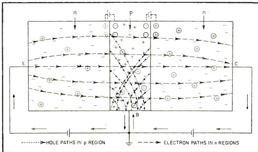
FIG. 4—Diagram of carrier paths for an *nnp* junction transistor. Conduction in *n* regions is by electrons; in *p* region by holes. Again dashed batteries simulate potential hills
