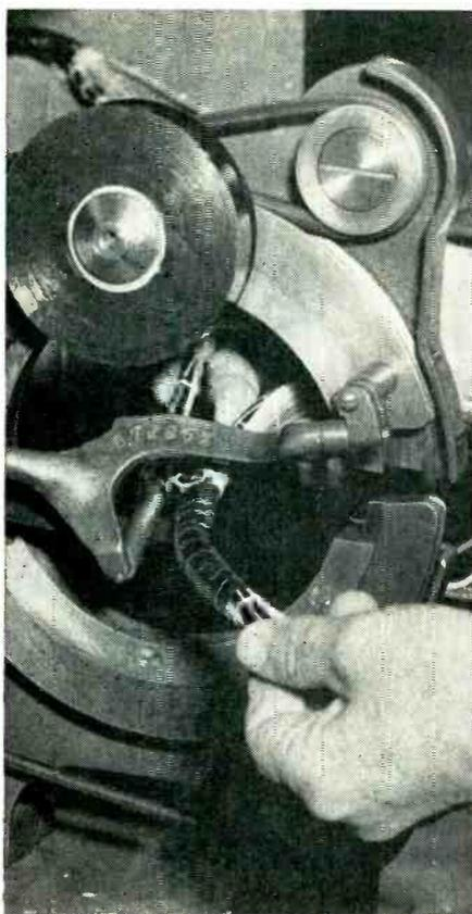
**INSULATING** a PECO rectifier harness calls for a compact tape with high dielectric. Here, *super-thin* "Scotch" Plastic Electrical Tape No. 33 neatly meets specifications. Has dielectric strength of 10,000 volts, yet is only 7 mils thick! Carries UL seal.
