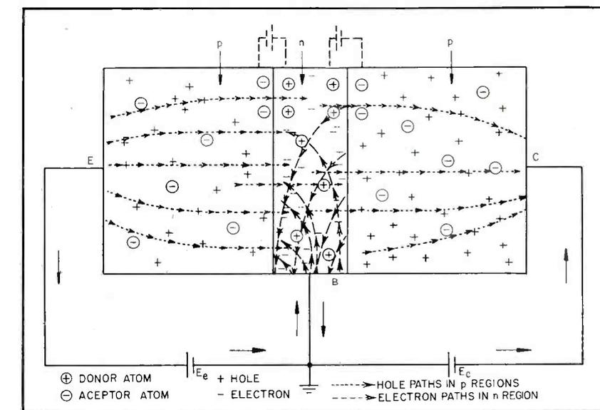
FIG. 1—Diagram of carrier paths in a pnp junction transistor show how conduction in  $p$  regions is principally by holes. Holes from emitter  $p$  region pass through base  $n$  region, suffer recombinations and complete circuit through collector  $p$  region. Base current is small because  $I_e$  and  $I_c$  flow in opposite directions as shown. Equivalent batteries (dashed) simulate effect of potential hills
