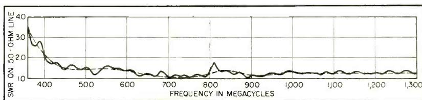
FIG. 5—Optimum parameters, standing-wave ratio versus frequency, for 60-degree discone
