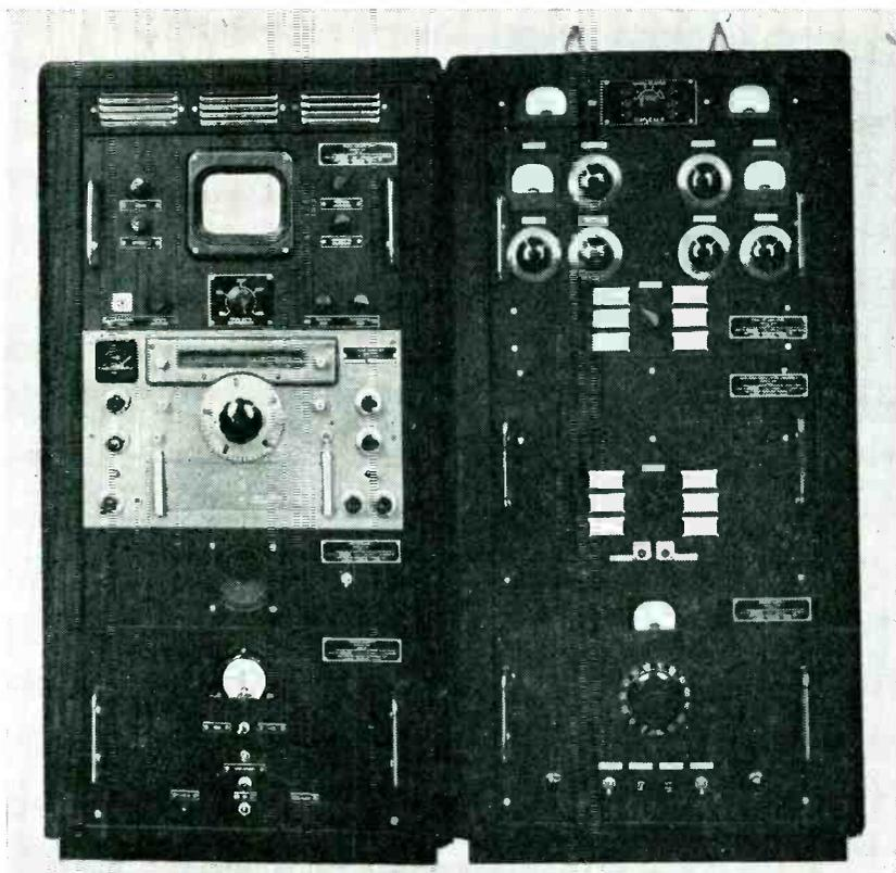
Communication Zone Indicator. Left-hand bay contains timing, indicating and receiving units. Transmitter and antenna duplexer are at right
