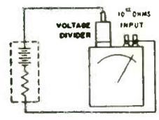
**CURRENTS AS LOW AS  $10^{-14}$  ampere** are measured directly with Model 2001 Electrometer shunts. Available with resistances from  $1.0 \times 10^6$  up to  $1.0 \times 10^{12}$  ohms. Typical uses: photocell currents (shown), ion chambers, capacitor and insulation leakages.
