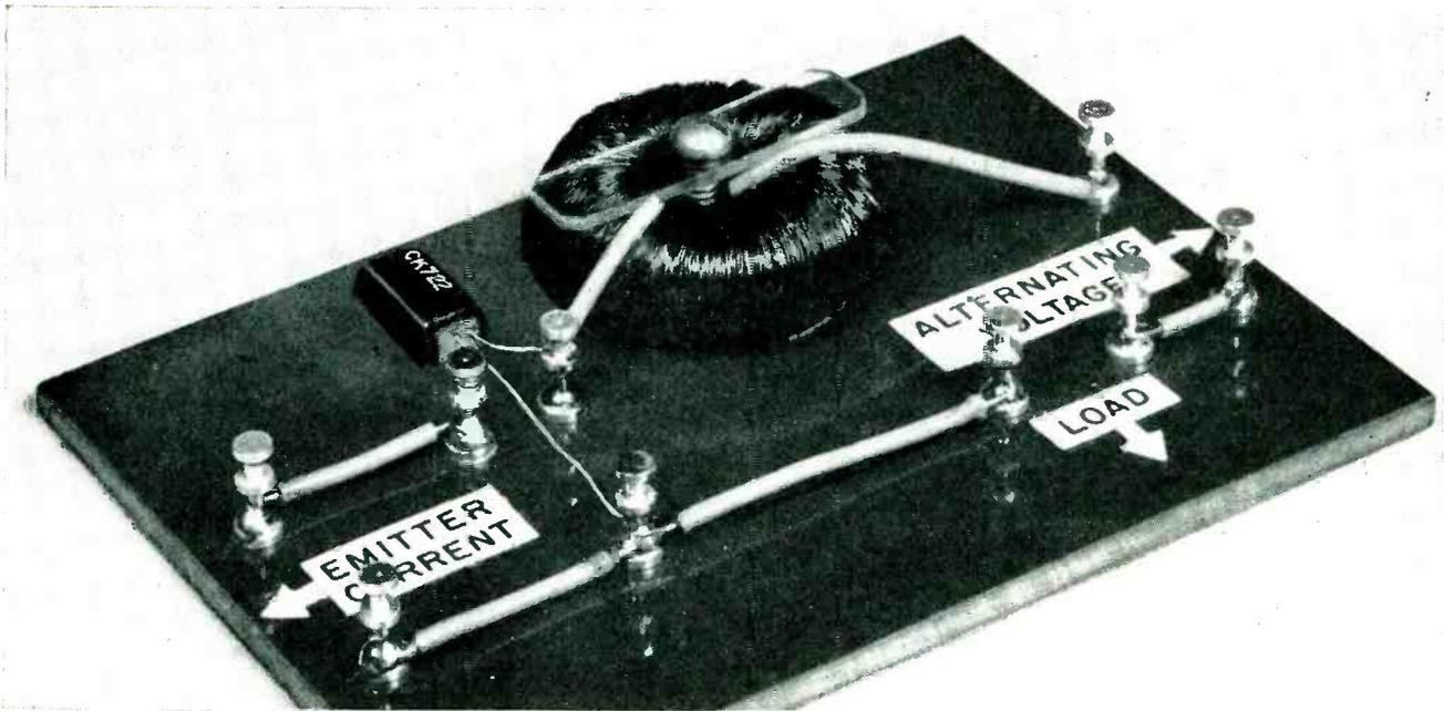
Experimental transistor-controlled magnetic amplifier using single-winding toroid with CK722 junction transistor. With 60-cps. 12.5-volt rms carrier voltage applied to terminals at right, output signal currents up to 100 ma peak can be obtained in connected load for emitter input signal currents under 0.5 ma peak
