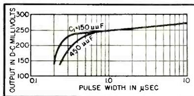
FIG. 6—Effect of pulse width with constant peak amplitude for two values of series capacitor
