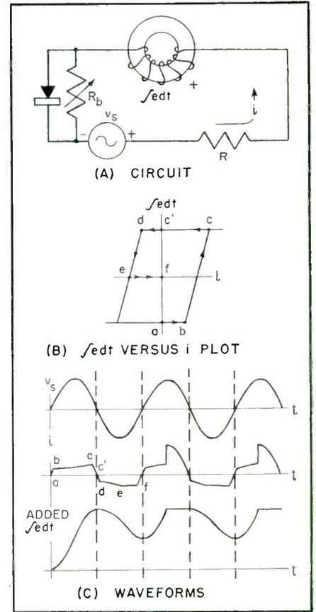
FIG. 4—Modified diode circuit using shunt rheostat to establish operating conditions between those of Fig. 2 and 3
