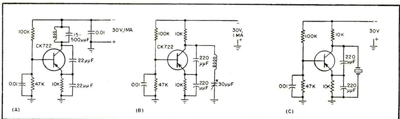
FIG. 5—Three typical transistor oscillators. Upper frequency limit depends, among other factors, on transistor used
