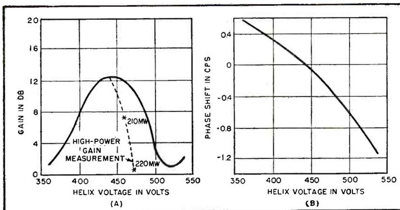
FIG. 4—Phase and gain versus helix voltage for oscillator using tube 14 wavelengths long
