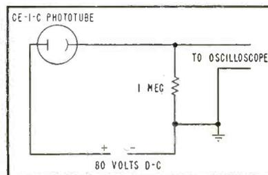
FIG. 1—Phototube circuit used to measure camera shutter speed
