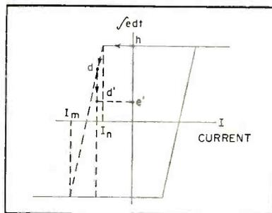
FIG. 9—Composite characteristic of magnetic core, illustrating behavior during reset half-cycle
