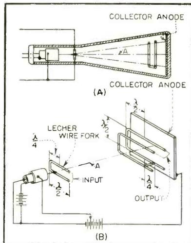
FIG. 1—Microwave energy amplifier tube (A) and circuit detail (B)
