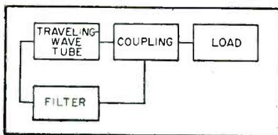
FIG. 1—Block diagram of traveling-wave-tube oscillator
