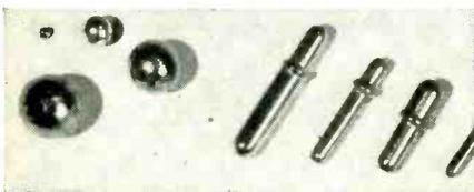
Multi-swage products — hollow tubular parts with tightly swaged seams — are widely used for contact pins, terminals, jacks, and sleeves. Friction fasteners made by this process retain their spring properties remarkably well. Courtesy The Bead Chain Manufacturing Co., Bridgeport, Conn.
