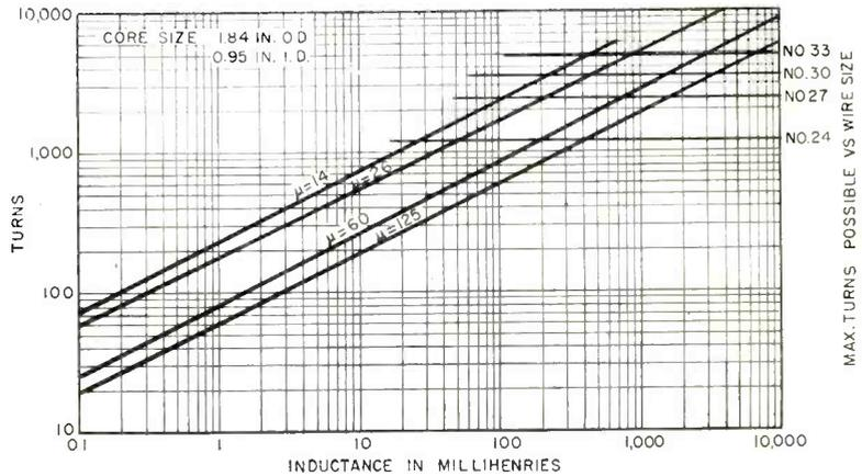
FIG. 1—Master design chart for toroids with 1.84-in. (O. D.) cores
