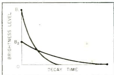
FIG. 3—Phosphor afterglow characteristics show that the phosphor having the shorter decay time must be operated at a higher initial brightness level,  $B_2$ .
