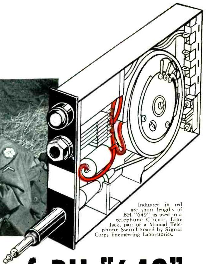
Indicated in red are short lengths of BH "649" as used in a telephone Circuit, Line Jack, part of a Manual Telephone Switchboard by Signal Corps Engineering Laboratories.
