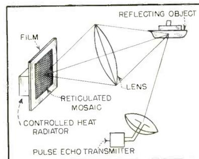
FIG. 11—Basic concept of radar photographic method by r-f reflection
