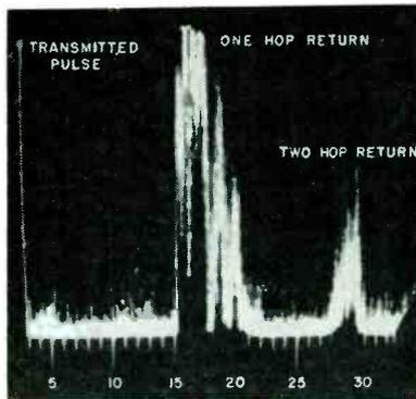
Range-scope presentation shows transmitted pulse and backscattered signals
