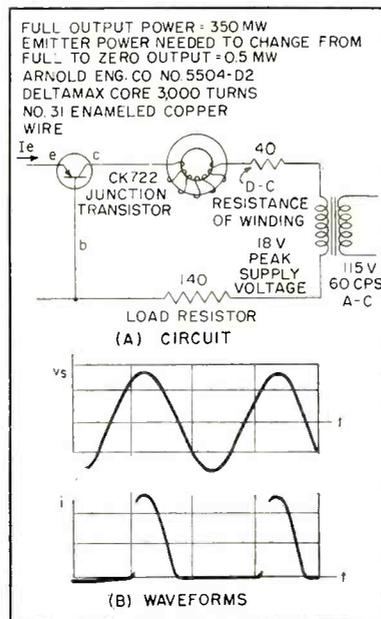
FIG. 6—Experimental version of final circuit, with waveforms of a-c supply voltage and load current
