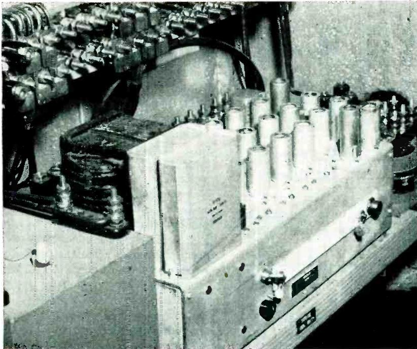
Sweep-frequency oscillator unit in concrete bungalow adjoining railroad tracks sweeps from 160 to 310 kc
