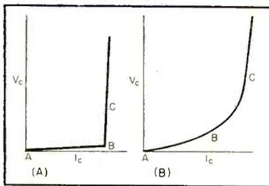
FIG. 2—In (A) is shown collector characteristic for junction transistor. Note very steep operating region at point C indicating high collector-to-base resistance. In (B), the point-contact characteristic, collector resistance of about 18,000 ohms at operating point C is indicated, compared with 1 megohm for junction type
