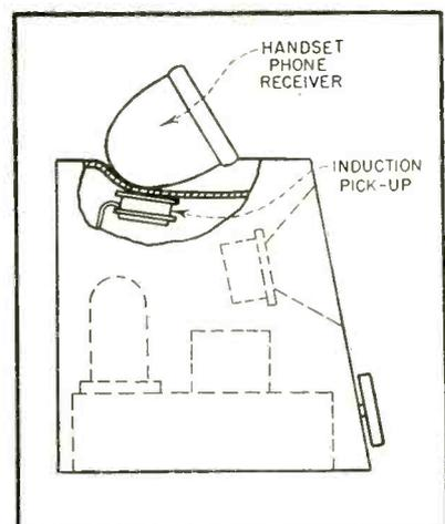
FIG. 8—Induction pickup obviates need for direct connection to telephone
