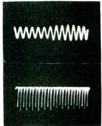
Sine-wave input at top, results in series of sharp negative peaks in the output
