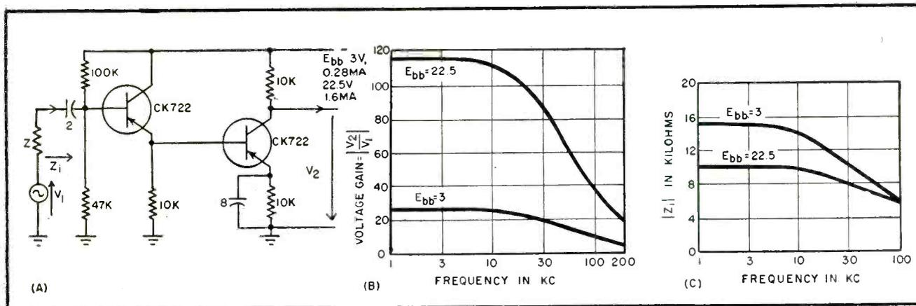
FIG. 2—Two-stage amplifier with high input impedance and direct-current stabilization
