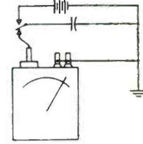
**EXCEPTIONALLY FAST** way to check capacitor leakage—by direct measurement of voltage decay. Also easily measured: piezo-electric potentials, vacuum tube electrode potentials, electrostatic fields.
