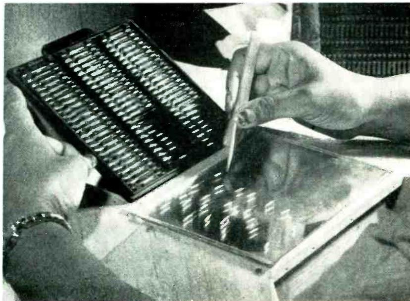
Mirror setup used for inspecting both sides of small parts simultaneously
