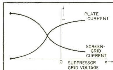
FIG. 3—Conduction shifts from screen to plate in pentode
