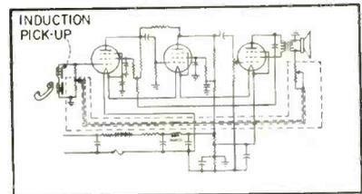
FIG. 7—Telephone amplifier features feedback
