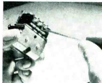
Using step gage to measure contact gap in aircraft relay
