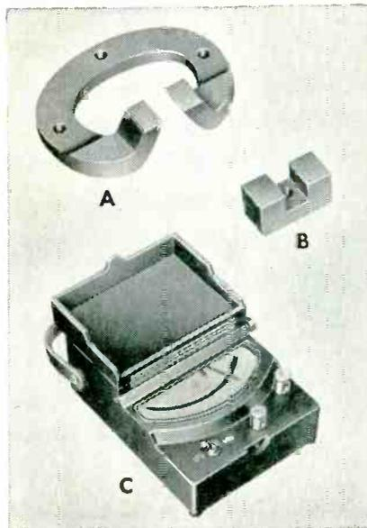
**Instruments**—Figure A is damping magnet once used in GE indicators. Figure B is tiny Carboloy magnet now used. It permits smaller indicator design (Fig. C), cuts materials and assembling costs . . . speeds up calibrations.
