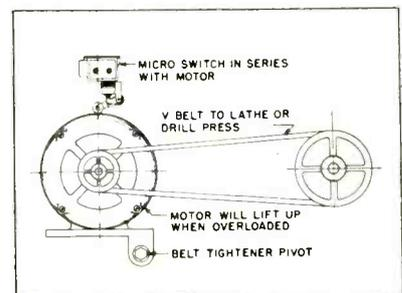
Method of using switch in place of fuse to break circuit when fractional-horse-power electric motor stalls
