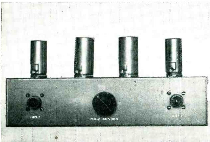
Front view of completed generator shows simplicity of construction. Channel-lock cabinet used is 10  $\times$  4  $\times$  2 $\frac{1}{2}$  in.
