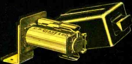
Clare Relays which perform precise functions in control of Sciaky welders are of plug-in type with dust covers
