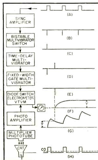
FIG. 1—Block diagram and associated waveforms show sequence of operations
