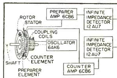
FIG. 4—Diagram of magnetic digitizer
