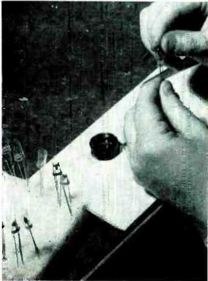
Placing sleeve over transistor. Units are stored in foam polystyrene block between operations
