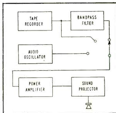
FIG. 2—Porpoise reaction tested with recorded sounds and single tone from audio oscillator
