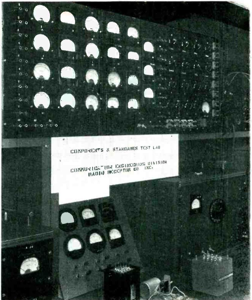
Portion of test facilities for type-approval of components. Patch cords are used to connect meter jacks at upper left with component under test on bench and simulated loads at center of panel. Universal power supplies are on bench
