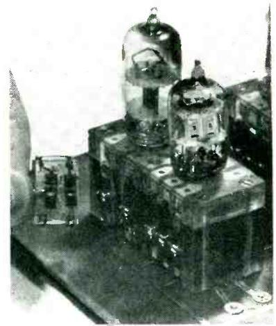
FIG. 1—Cellular technique for mechanized wiring employs three-terminal molded cells that fit into two-tube building block. Printed wiring is used on base plate. Extensions of tube-socket springs make contact and hold blocks in place
