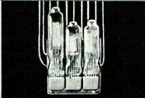
**New Sub-miniature Model III Ampec** — a full three-stage speech amplifier of remarkably small dimensions — approximately 1 1/32" x 1 1/16" x 1 1/32" (barely larger than a postage stamp!). Excellent for microphone preamplifiers and similar applications. Check No. 42-130 on coupon for complete information.
