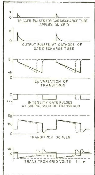
FIG. 4—Waveforms encountered in transitron sweep circuit
