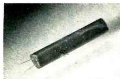
Polyethylene foam surrounds two copper-clad steel wires. Trapped gas bubbles improve the characteristics of this new uhf-tv lead-in that requires no taping or sealing and works equally well in dry or wet weather
