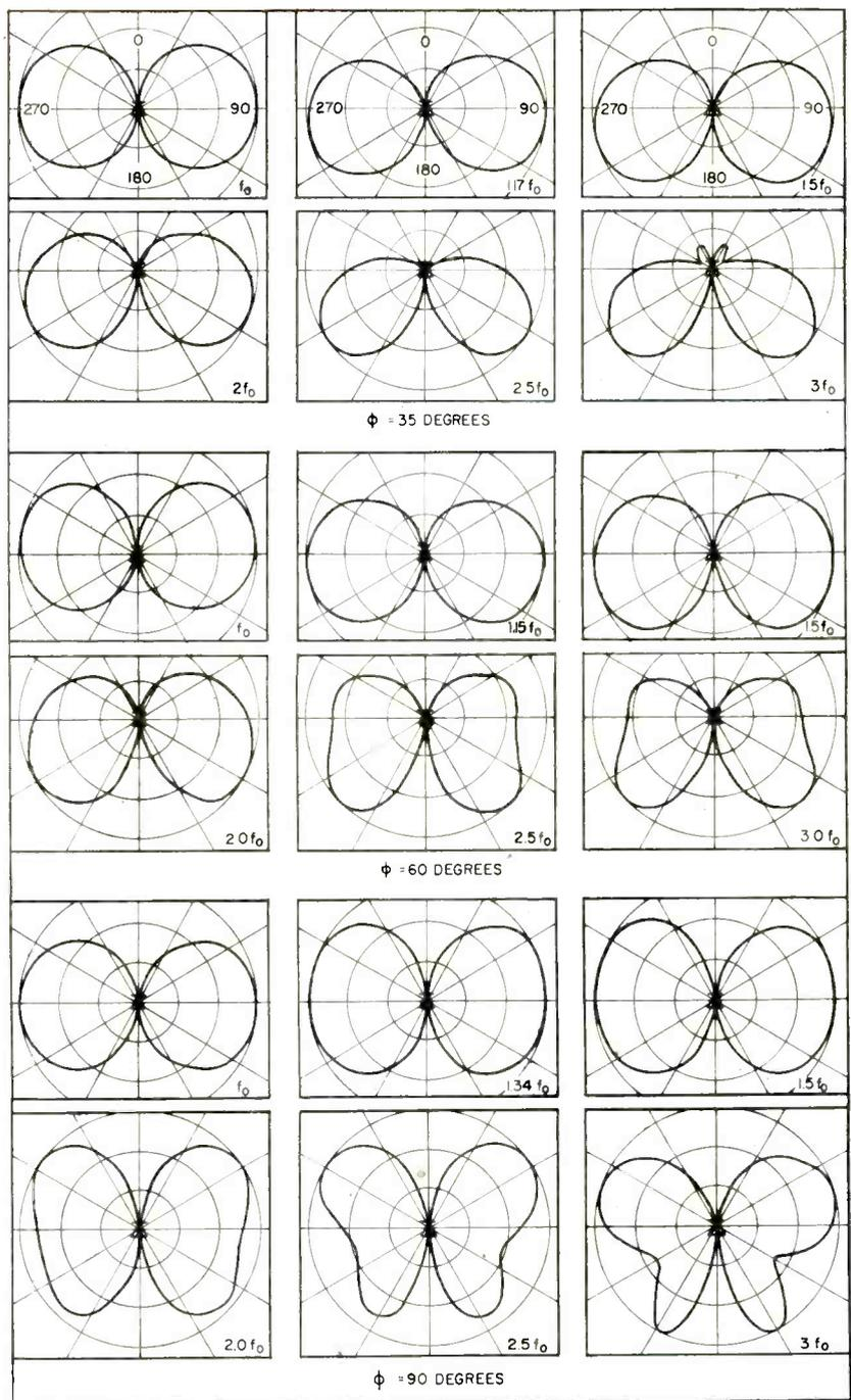
FIG. 7—Relative E-plane normalized field patterns for different angles of  $\phi$
