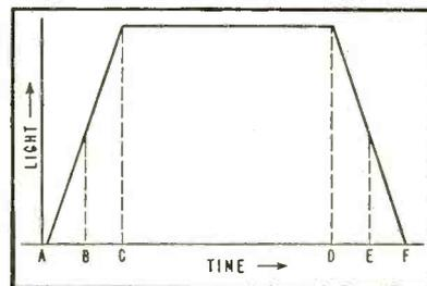
FIG. 2—Light passes through camera shutter during exposure. Slopes AC and DF are values during the opening and closing of the shutter
