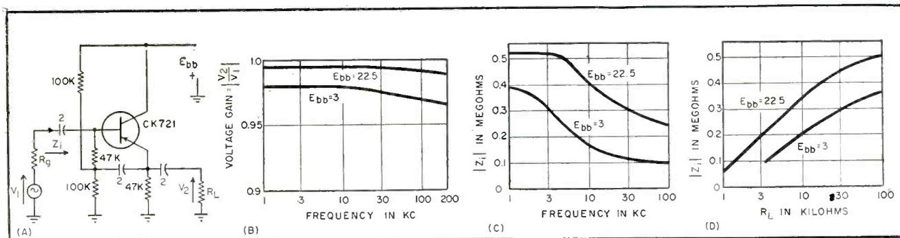
FIG. 3—Grounded-collector stage has high input impedance and low output impedance. Voltage gain approaches unity
