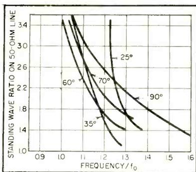
FIG. 3—Standing-wave ratio versus ratio of lowest operating frequency to  $f_0$  when  $f_0$  is frequency at which slant height is a fourth wavelength
