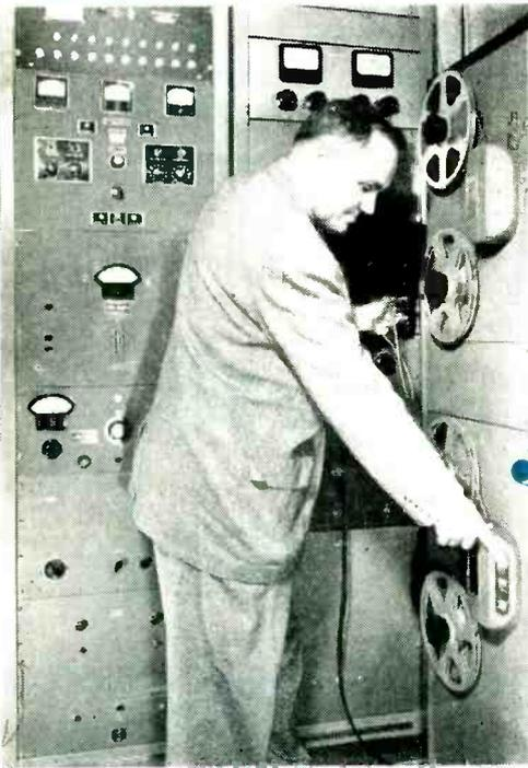
An Ampex Automatic Station now in operation at KEAR in San Mateo, California. It sustains the evening programs on tapes prepared by the daytime staff.
