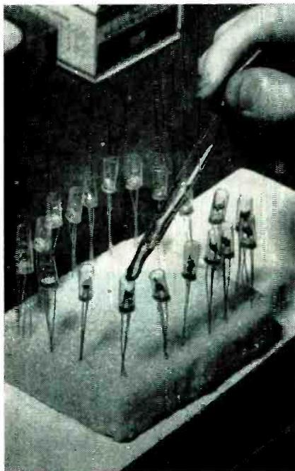
Using medicine dropper to fill each transistor sleeve with potting resin
