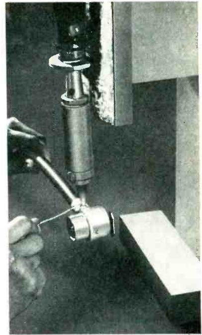
Vertical support for soldering iron used in soldering ferrules of cable shield to shell of connector plug
