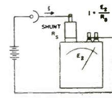
**RESISTANCES UP TO  $10^{16}$  OHMS** are easily measured with Wheatstone Bridge circuit diagramed, or by measuring current resulting from known applied voltage. Typical uses include: standardizing resistors, measuring insulation samples.
