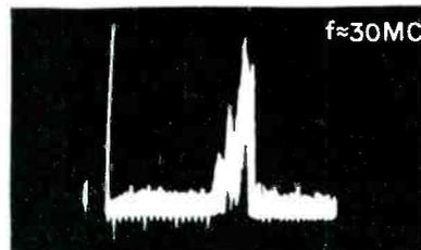
Presentations of backscatter, showing increase in skip distance as transmitter frequency is increased
