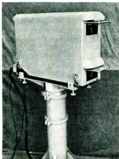
Detector portion of unit transmits and receives light beams
