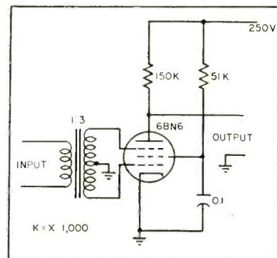
FIG. 1—Gated-beam tube zero-crossing detector uses push-pull connection on two grids to keep tube cut off except in zero-voltage region
