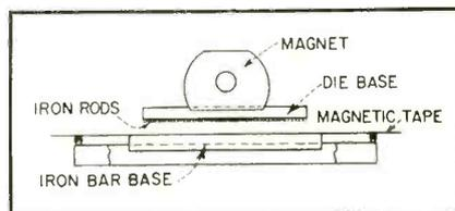
FIG. 5—Printing die for impressing magnetic pattern on tape
