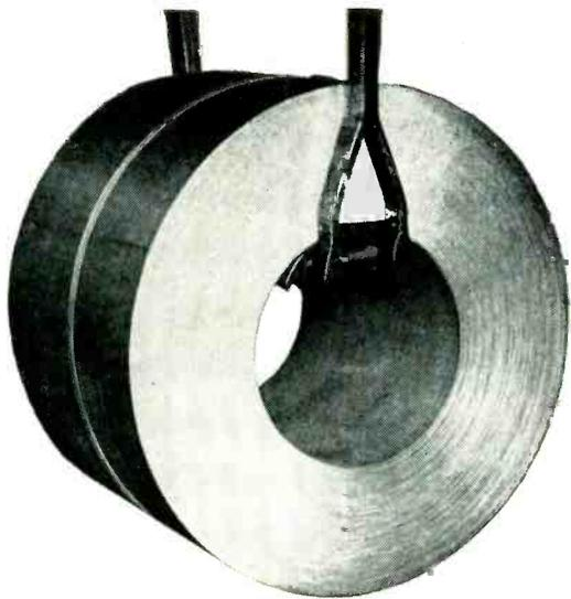
Long coils of DI-MAX Quality permit continuous press operation, eliminate end-of-sheet scrap losses.
