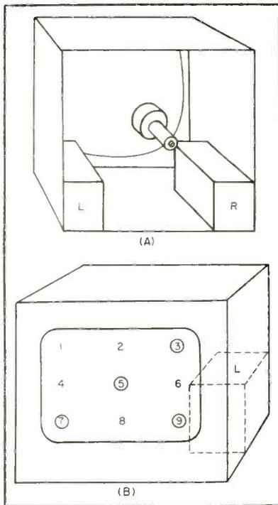
FIG. 1—Sketches show optimum location for power transformer in table-model tv receiver (A) and spots on cathode-ray tube studied in tests (B)
