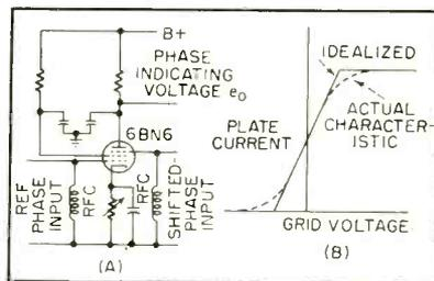
FIG. 1—Simplified phase detector (A) and plate-current limiter-grid voltage curves for 6BN6 (B)
