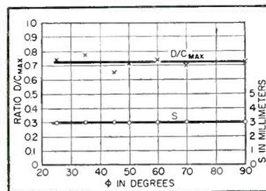
FIG. 2—Optimum values of disk-to-cone spacing and disk diameter versus flare angle
