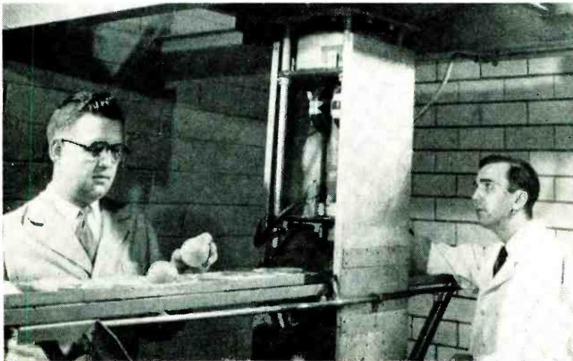
Converted x-ray machine used to produce electron stream. Experiments now in progress show that cold sterilization and prevention of spoilage may be possible by lethal effect of cathode rays on insects, bacteria and mold. Test have already been conducted, with apparently favorable results, on oranges, bread and minute steaks
