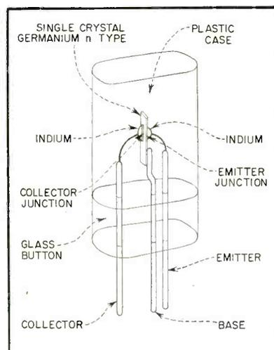
Artist's drawing of inside of typical *pn*p junction transistor made by diffusion or alloy process
