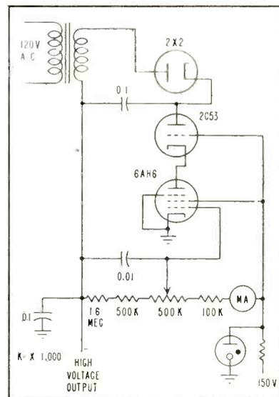
FIG. 1—Circuit of high-voltage power supply
