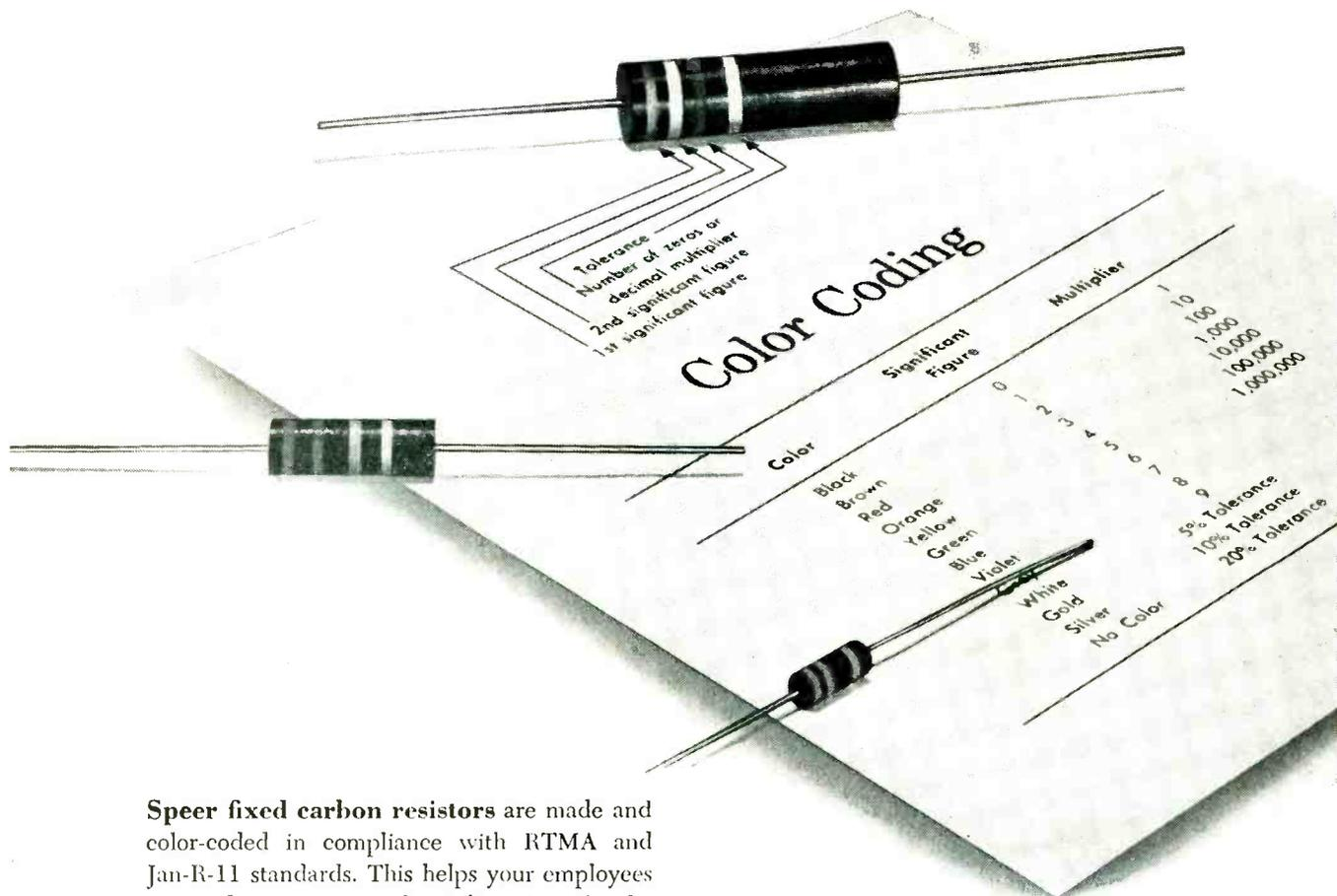
**Speer fixed carbon resistors** are made and color-coded in compliance with RTMA and Jan-R-11 standards. This helps your employees to avoid errors—to use the *right* resistor for the circuit every time.
