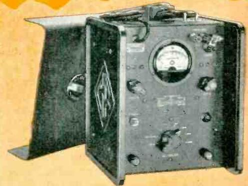
Insulation Resistance is measured directly by the Type 1862-A Megohmmeter at the commonly accepted ASTM potential of 500 volts.
