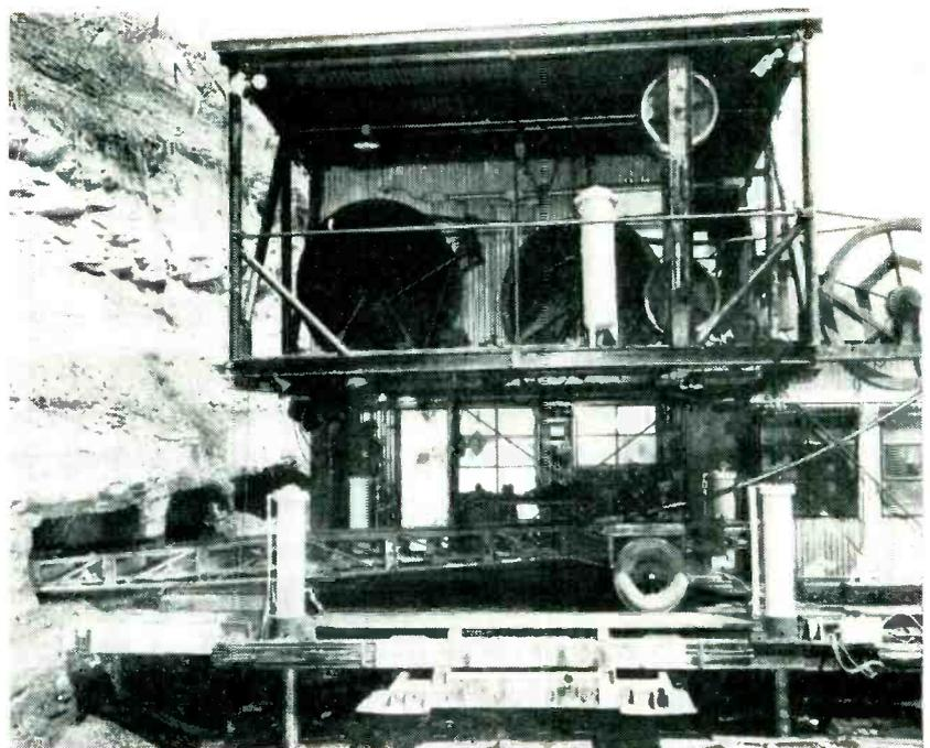
Mining machine, with cutter and front end of first portable conveyor already underground at start of new tunnel. Power and control cables, stored on large upper-deck reels, ride in L-shaped hooks at far side of conveyor. Windows of control station can just be seen at right on machine
