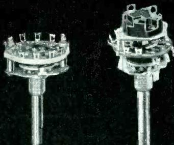
**For miniature switches** — specify Centralab's Series 20 with Steatite or Phenolic sections. Steatite is Grade L5. Meets JAN I-8 specs. Phenolic sections conform to JAN P-13 ... Grade LTSE4. Available in 2 to 11 positions with stops, or 12 positions, continuous rotation—single or multiple sections—with or without attached on-off switch. Check No. 42-156.
