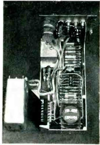
**G-E TANTALUM** capacitors installed in telephone carrier amplifier.
