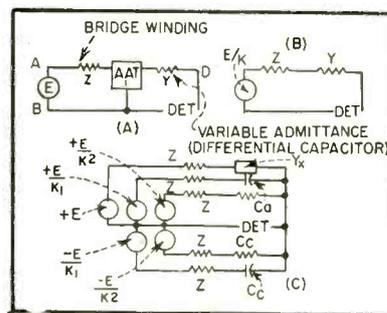
FIG. 10—Equivalent circuit (A) of left side, circuit with attenuator removed (B) and equivalent circuit of entire bridge (C)
