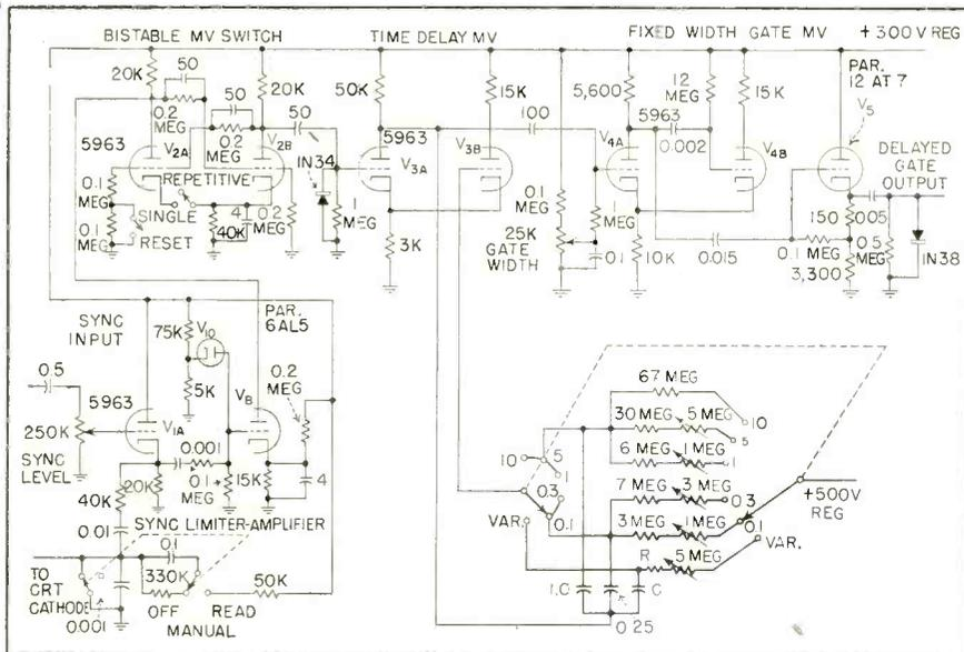
FIG. 2—Complete circuit of sync limiter-amplifier and multivibrator chain
