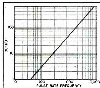
FIG. 7—Effect of pulse rate frequency on output
