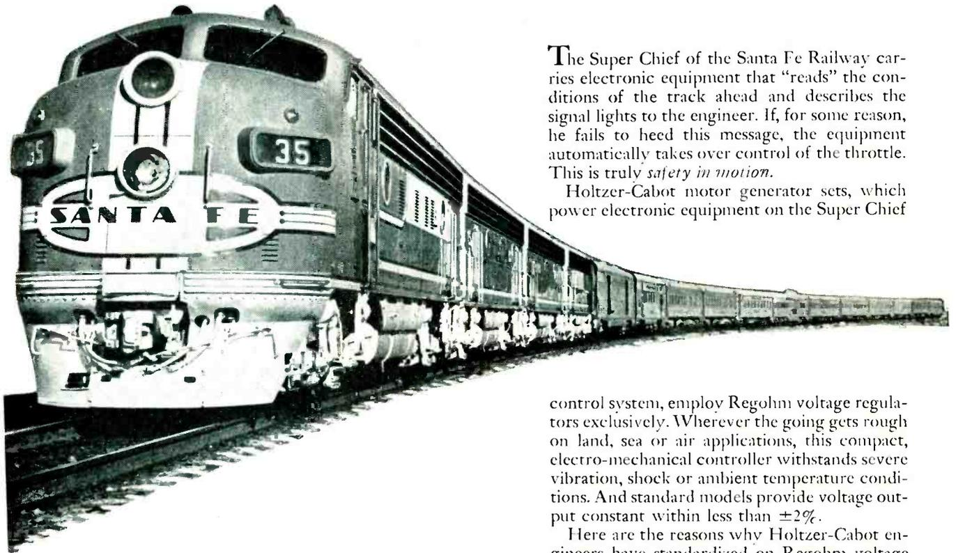
The Super Chief of the Santa Fe Railway carries electronic equipment that "reads" the conditions of the track ahead and describes the signal lights to the engineer. If, for some reason, he fails to heed this message, the equipment automatically takes over control of the throttle. This is truly *safety in motion*.
