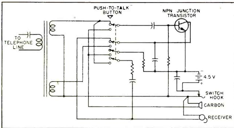
FIG. 3—High-efficiency railroad dispatcher's telephone subset uses junction transistor
