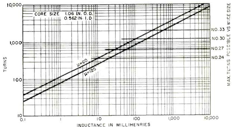
FIG. 2—Master design chart for toroids with 1.06-in. (O. D.) cores
