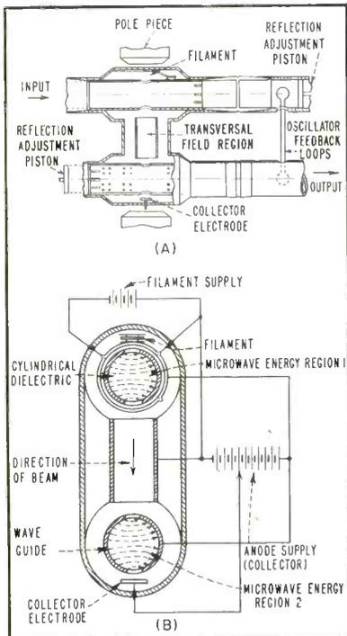
FIG. 14—Physical structure (A) and field regions (B) of special klystron
