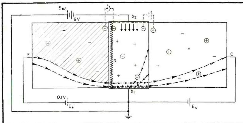
FIG. 6—Transistor tetrode operation depends on added field supplied by battery connected to side of base opposite usual base connection. Added field bunches electrons in emitter region. Equivalent batteries simulate potential hills, and resistance  $R$  represents uniform voltage divider within base region from top to bottom of germanium bar
