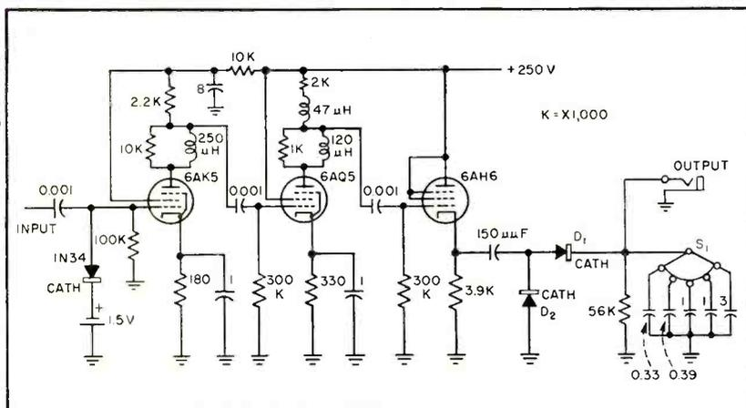
FIG. 3—Pulse-averaging voltmeter circuit
