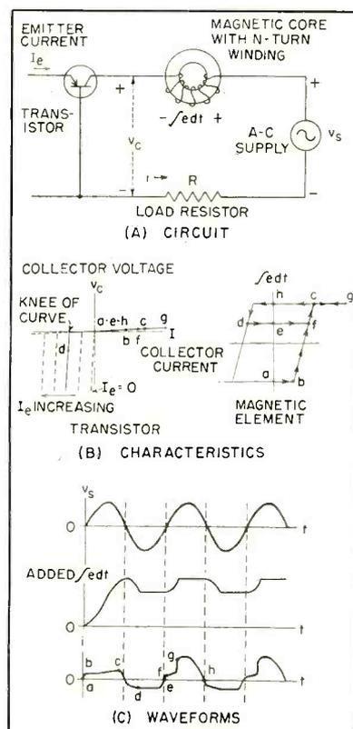
FIG. 5—Operation of transistor-controlled magnetic amplifier circuit
