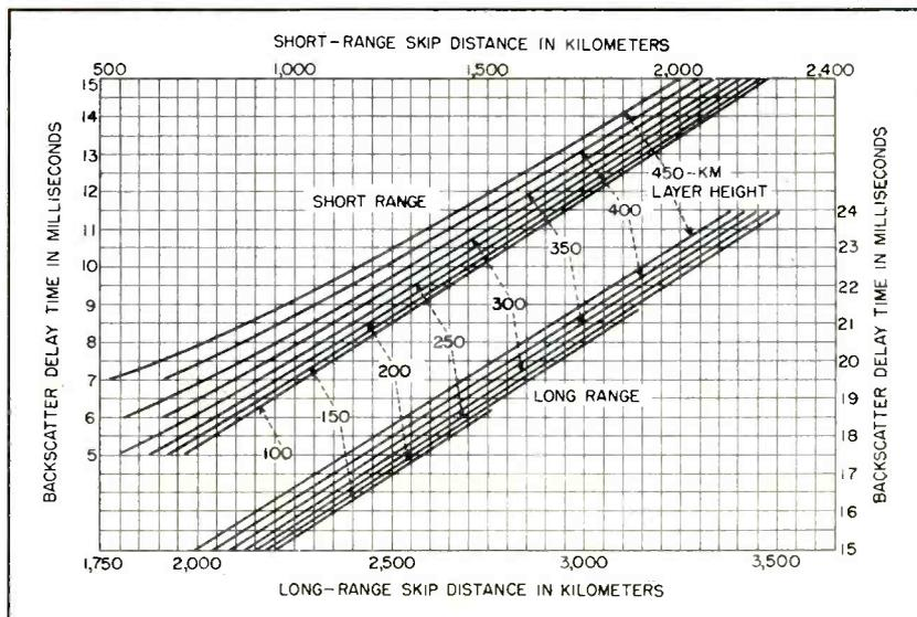
FIG. 1—Conversion chart used to obtain skip distance from time delay between transmitted pulse and reception of backscattered signals
