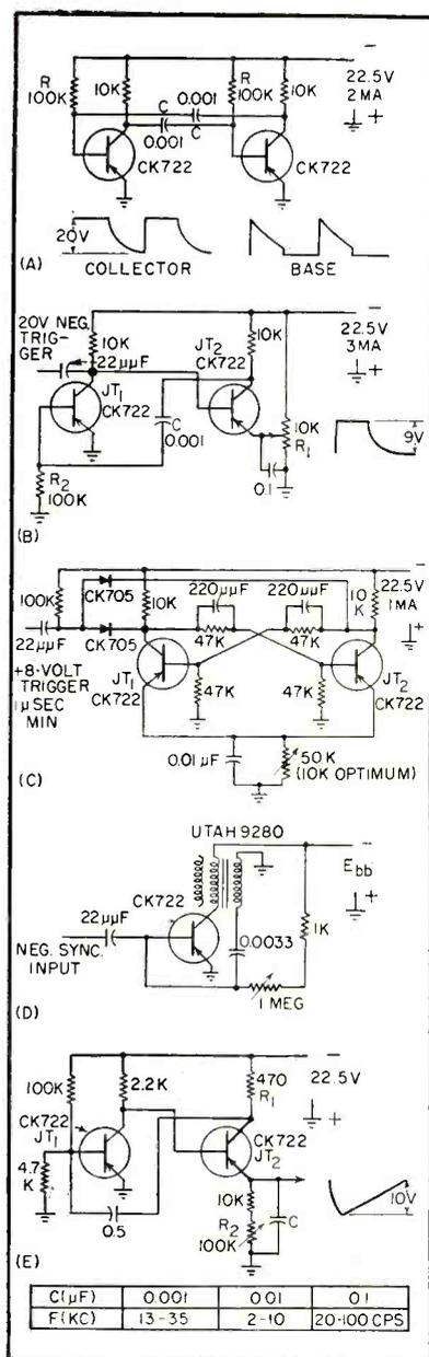
FIG. 6—Pulse circuits include an astable multivibrator (A), monostable multivibrator (B), bistable multivibrator (C), blocking oscillator (D) and transistorized version of Puckle's sweep circuit (E)
