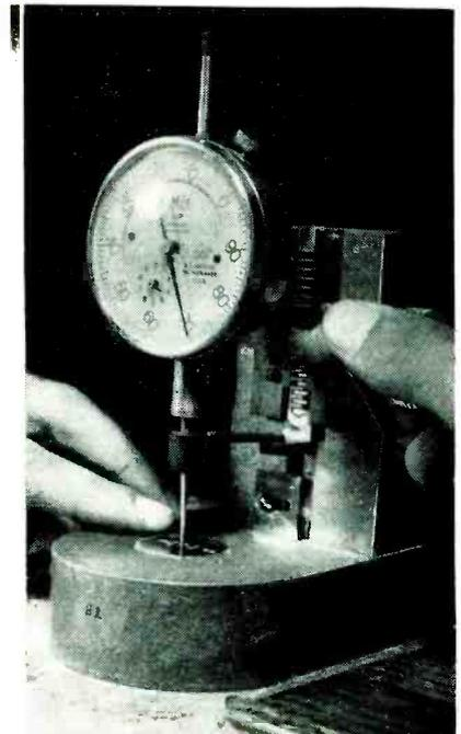
Operator here is rotating knurled knob clockwise with right hand to lower spindle, for gaging diameter of center hole in mica spacer
