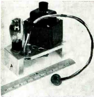
Power sub-chassis helps to isolate power-frequency fields in an export tv set
