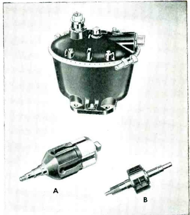
**Magnetos** — To save space and weight, Scintilla Magneto Division, Bendix Aviation Corporation, now makes aircraft magneto rotors from Carboloy permanent magnets. Figure A shows old-style rotor that weighs 4 lbs. 9 ozs. Figure B shows new rotating Carboloy permanent magnet weighing only 2 lbs. 4 ozs. — less than half as much as old-style rotor.
