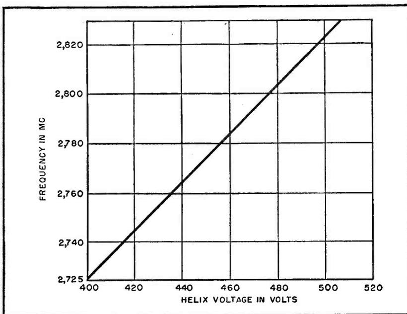
FIG. 5—Tuning curve for oscillator using 14-wavelength traveling-wave tube
