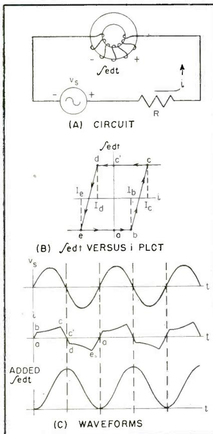
FIG. 2—Simple series circuit using magnetic core. Only small magnetizing current flows
