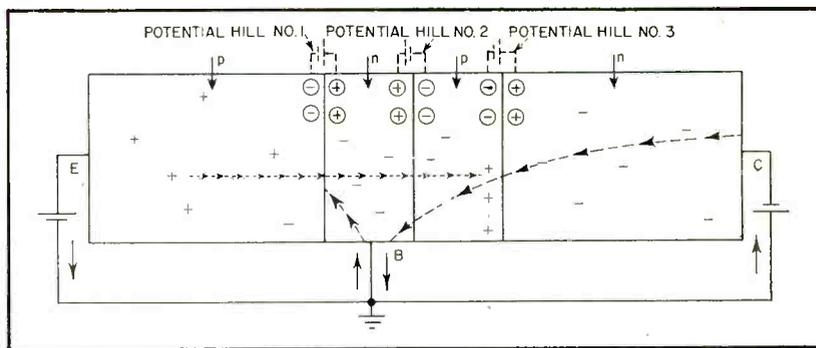
FIG. 7—Simplified diagram shows operation of *pnpn* hook transistor. Current gains of more than 20 have been exhibited by this type
