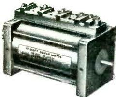
**FORD SERVO MOTORS** (60 and 400 cycles) for extremely low inertia and high frequency response. 1/5; 1/2; 1 1/2; 2 1/2; 5; 10-watt models in both low and high voltage, including magnetic amplifier controlled types.
