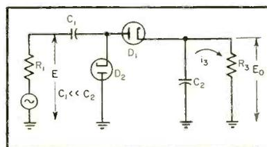
FIG. 1—Basic voltmeter circuit
