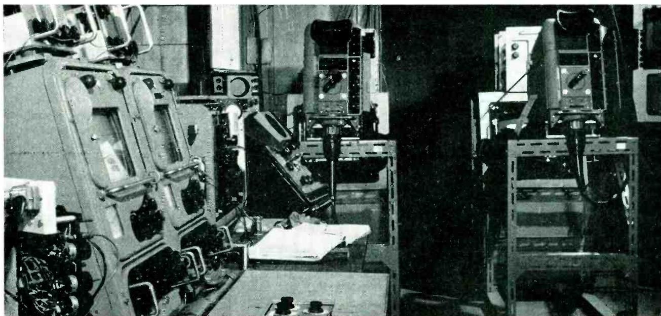
Equipment for converting between French 819-line standards and British 405-line standards is located at Cassel in northern France. Twin standards converters are at right with monitor console, left. Television scenes of coronation ceremony were routed through Cassel via microwave links to feed a five-nation television network
