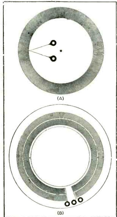
FIG. 3—Rotor (A) and stator (B) patterns for magnetic shaft-position digitizer
