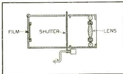
FIG. 12—Arrangement of camera for radar photography
