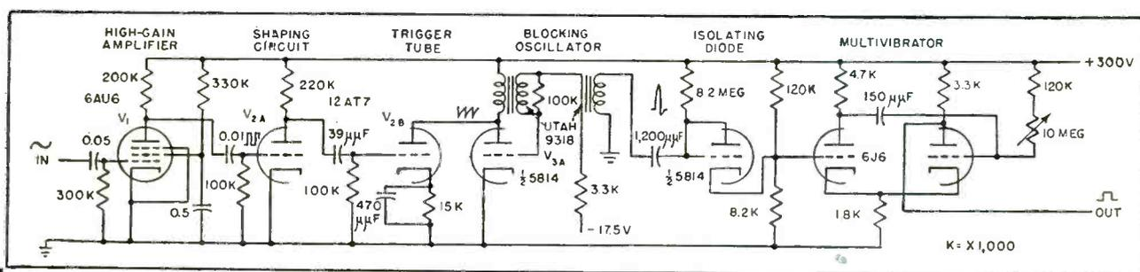
FIG. 1—Circuit diagram of variable-length pulse generator. Power requirement, exclusive of filaments, is about ten watts; regulated B+ and bias supplies are recommended
