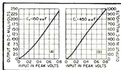
FIG. 5—Amplitude characteristics for two values of series capacitor in Fig. 1 and 2
