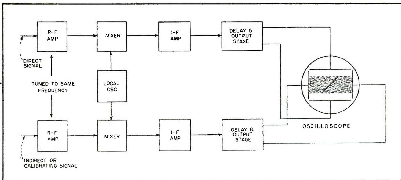
FIG. 2—Twin-channel superhet and crt oscilloscope provide one-to-one Lissajous pattern to detect and measure signals with poor signal-to-noise ratio
