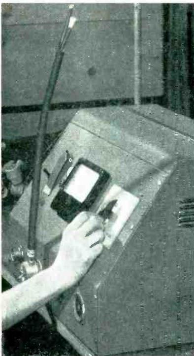
Using insulation resistance test set directly for checking one cable at a time. Operator's hand is on zero-adjust knob. Metal strip at left on panel prevents operator from moving one of the toggle switches accidentally
