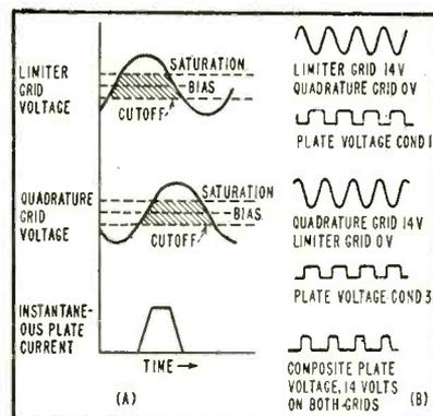
FIG. 2—Predicted waveforms (A) and reproductions of crt waveforms (B)
