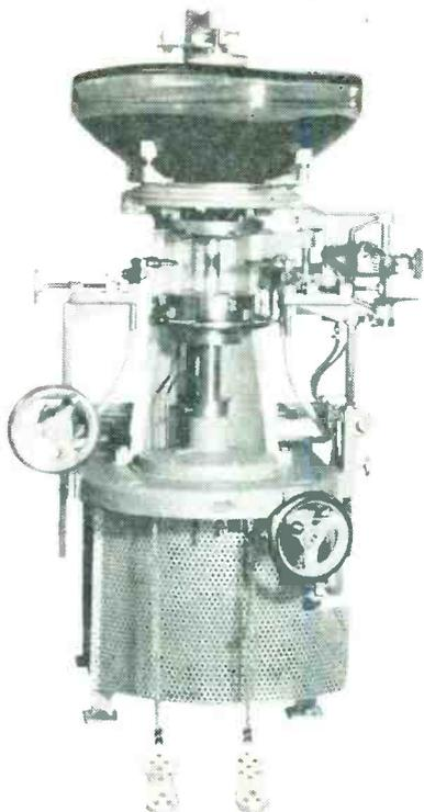
Machine for putting new neck on rejected picture tubes ranging up to 33 inch in size and even larger
