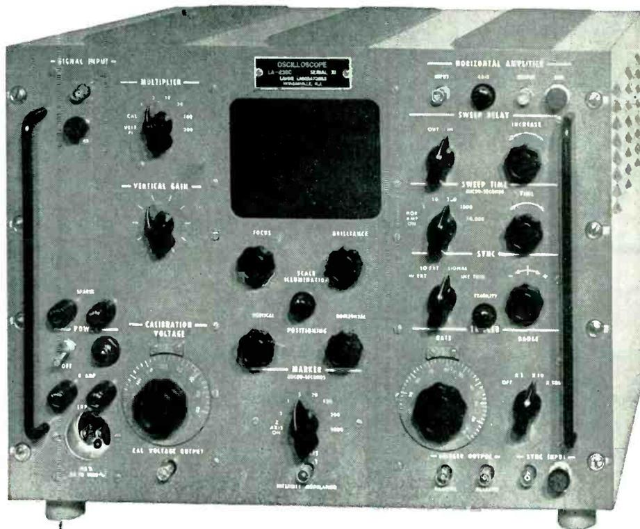
**THE LAVOIE MODEL LA-239C** has been designed to surpass the high performance of the TS-239A/UP, which has been the standard test oscilloscope for the Armed Services since its introduction. Model LA-239C is the result of a long period of research and development which has included the study of new tubes, new circuits, and new techniques. Rugged design has been combined with functional simplicity to produce an instrument as attractive as it is efficient.
