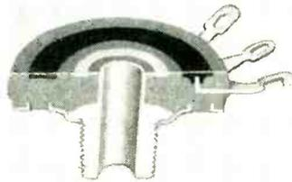
During manufacture, the molded resistor can be varied in resistance throughout its circumference. After molding, it is unaffected by temperature or moisture.
