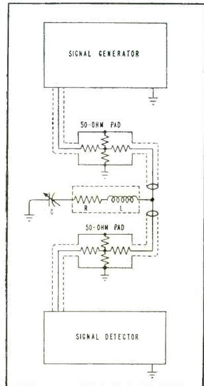
FIG. 2—Parallel connection of the measuring circuit used when unknown resistance is small compared to the 50-ohm pads
