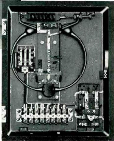
**PERFECT PERFORMANCE**, even after months of inoperation, is required of the electrical control unit. To meet this very severe and unusual operating condition, Ward Leonard 110 and 130 relays shown here give trouble-free performance with little or no maintenance. The midget 110 relay will open or close circuits up to ten amperes. The two-pole 130 relay can be economically adapted to a variety of applications by varying interchangeable parts in its assembly.
