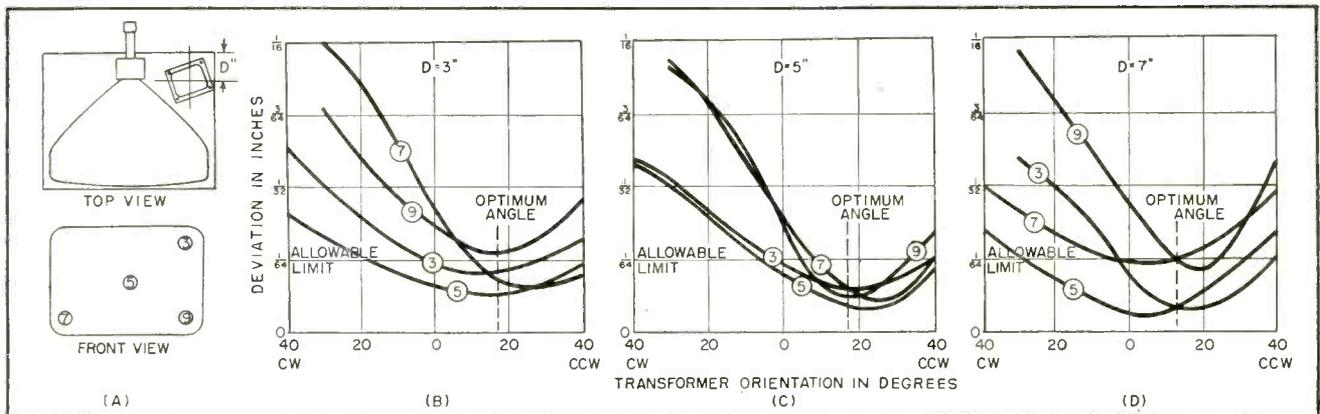
FIG. 2—Curves show effect of placement of power transformer on interaction between power-line and electron beam
