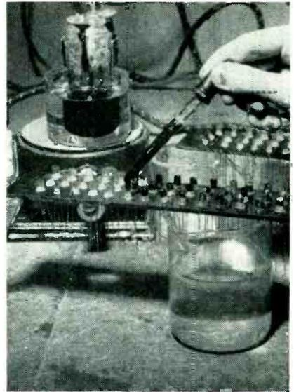
Potting germanium diodes with mixture of resin and lampblack, kept at 120 C with an oil bath on hot plate in background. Beaker in foreground merely serves as support for plastic strip holding diodes
