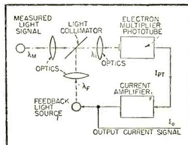
FIG. 1—Block presentation of the feedback photometer
