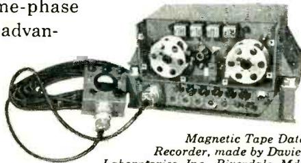
Magnetic Tape Data Recorder, made by Davies Laboratories, Inc., Riverdale, Md. uses Brush Magnetic Heads for Accurate Recording.
