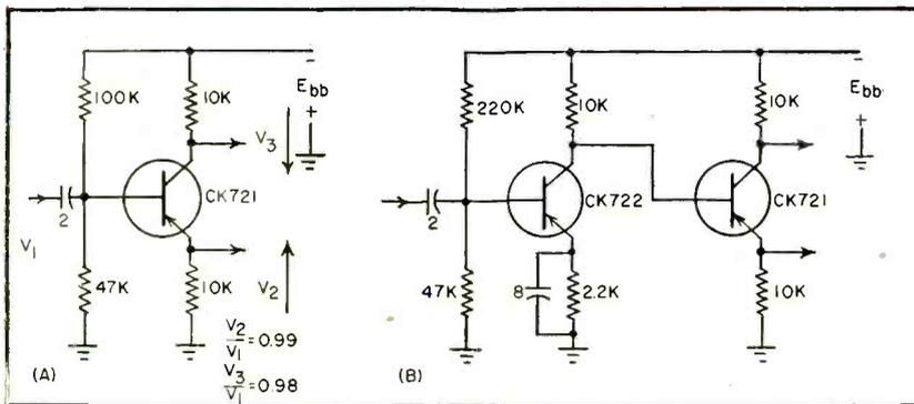
FIG. 4—Basic phase inverter (A) and phase inverter with amplifier
