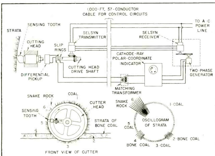
FIG. 2—Electronic control system for steering cutter accurately, at predetermined distance from roof or floor of wavy, wandering coal vein, for distances up to 1,500 feet in from control station
