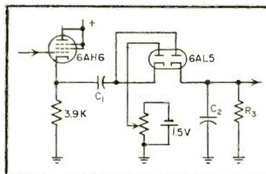
FIG. 2—Circuit using vacuum diode
