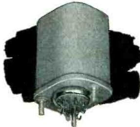
**RB 45 SERIES**—Similar to R 45 with the exception that it is designed to fit the hermetically sealed enclosure shown. Three stud mounting; solder terminals. Available up to 4 pole double-throw. Widely used in aircraft and ground communication equipment. Size: 1-5/8 x 1-7/16x2-1/32 D.
