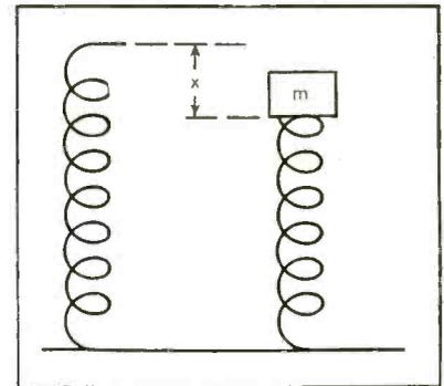
FIG. 1—Simplified concept of chassis and springing used in setting up equation for finding resonance of mounting springs
