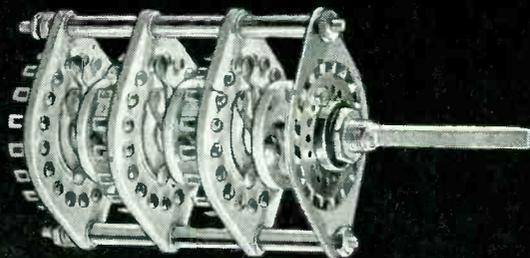
**Centralab's Medium-Duty Power Switches.** Use for R. F. or 110-115 V. application ... 7½ amps. Voltage breakdown to ground — 3000 volts—RMS 60 cycles. Available with Grade L5 (JAN I-8) Steatite sections — shorting or non-shorting contacts. Models in 1, 2 or 3 poles, 18 contacts per section with adjustable stops, can be furnished up to 20 sections per shaft. Contacts and collector rings are coin silver. For complete data, check No. 42-136 in coupon.
