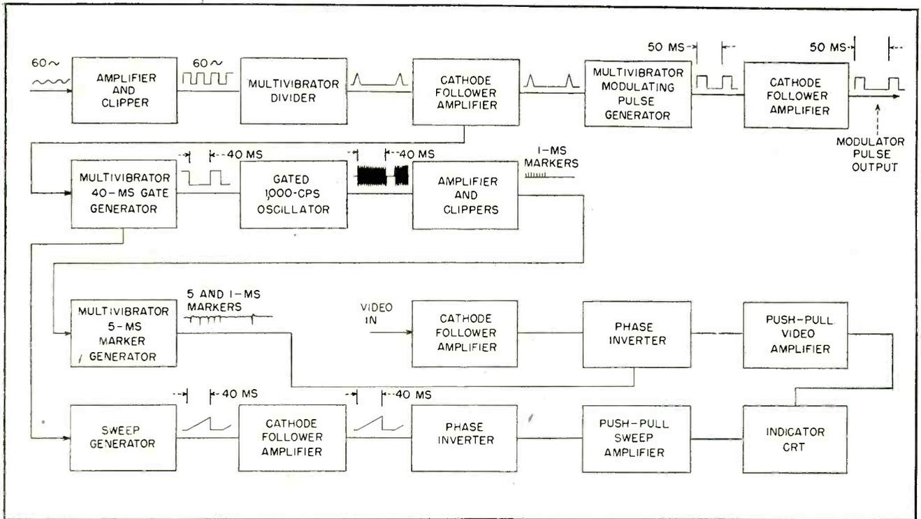
FIG. 3—Block diagram of timing and indicating circuits
