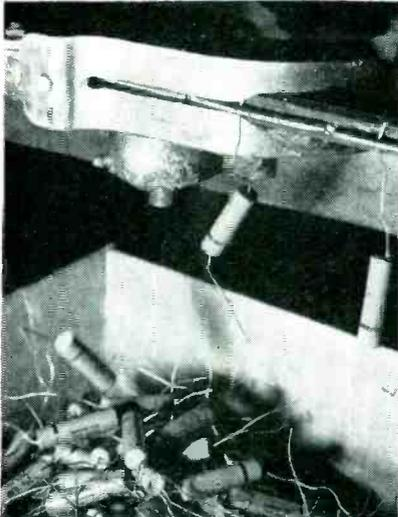
Claw-type device for removing dipped capacitors from coil spring as the spring moves from right to left through the claws
