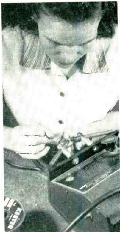
Method of using resistance-soldering unit to heat relay armature terminal for critical soldering operation
