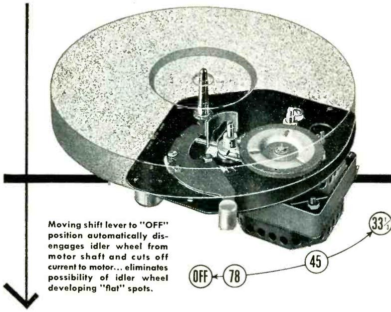
Moving shift lever to "OFF" position automatically disengages idler wheel from motor shaft and cuts off current to motor... eliminates possibility of idler wheel developing "flat" spots.
