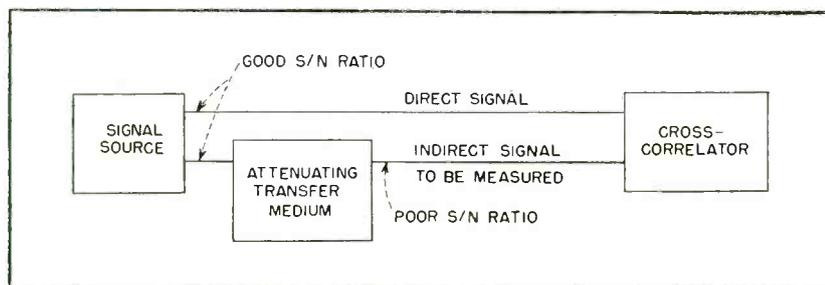
FIG. 1—Basic components of a cross-correlation system
