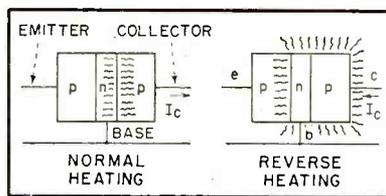
FIG. 8—Nature of power dissipation in a junction transistor
