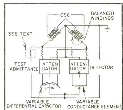
FIG. 9—Impedance measurements depend upon bridge circuit
