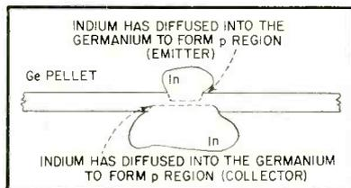
FIG. 3—Essentials of diffusion process for manufacturing *pnp* junction transistors are shown. Undiffused portion of indium (or gallium) dot is used to make appropriate connection
