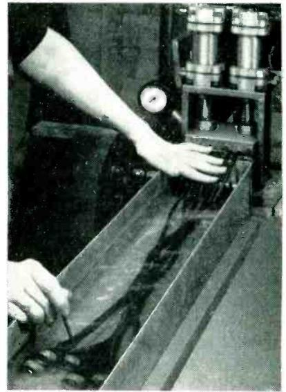
Setup using two air cylinders and longer trough for checking submerged cables for air leaks
