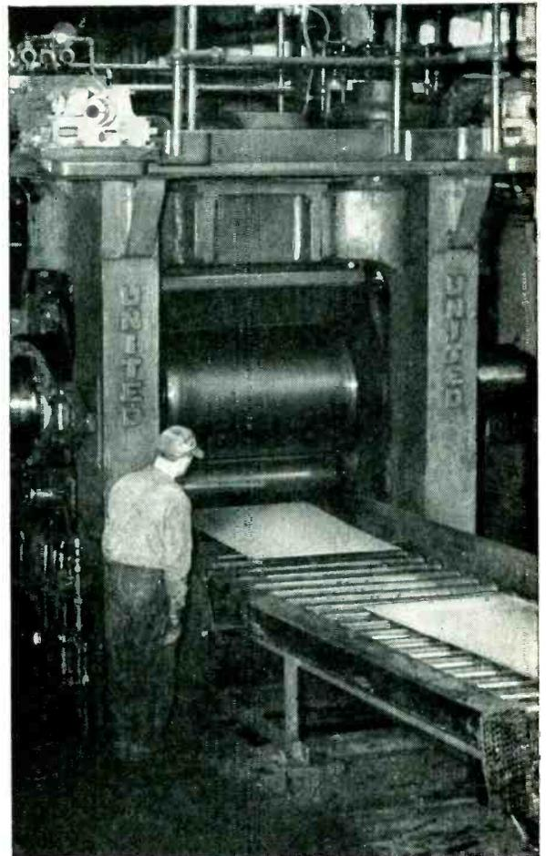
High pressures developed by four-high cold-finishing mills improve lamination factor in stacked cores.
