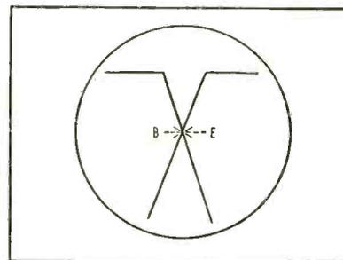
FIG. 3—Oscilloscope sweep is adjusted so points B and E on light curve will overlap
