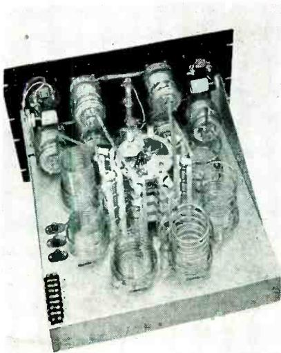
Transmitter final amplifier uses single 4-250A tetrode
