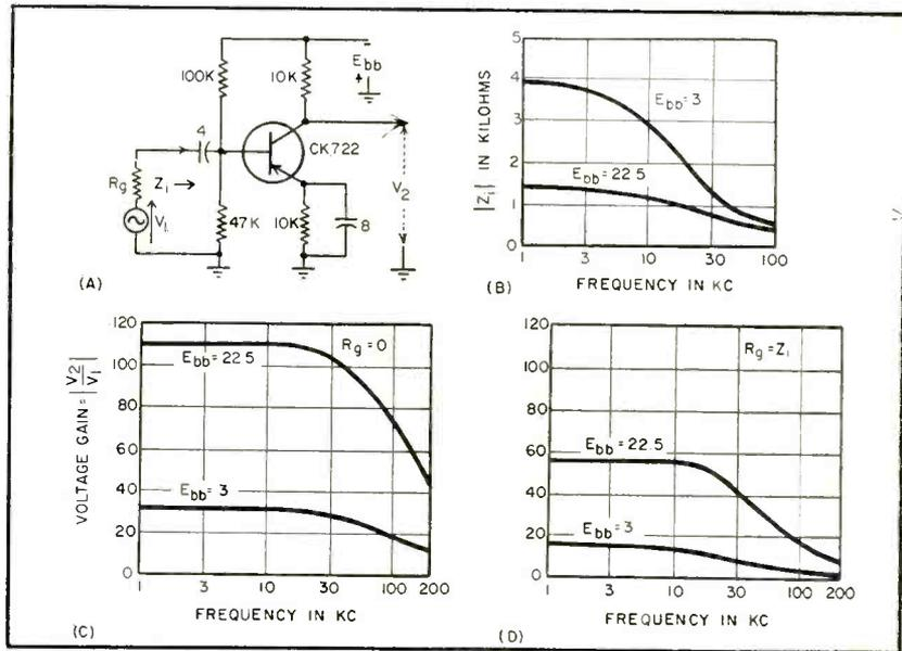
**FIG. 1**—Voltage amplifier using d-c stabilized grounded-emitter circuit is shown in **A**. Curves show circuit operating characteristics
