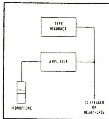
FIG. 1—System used to record porpoise sound on magnetic tape
