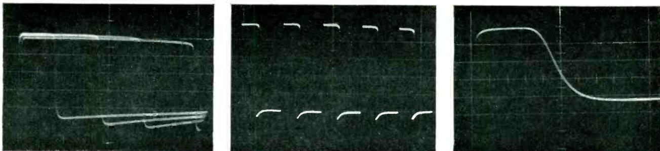
Control of pulse-length adjustment is illustrated at left by pulses of 2, 4½, 7 and 10 μsec. At center are 50-μsec pulses at 10 kc and a 0.5 μsec pulse at 20 kc
