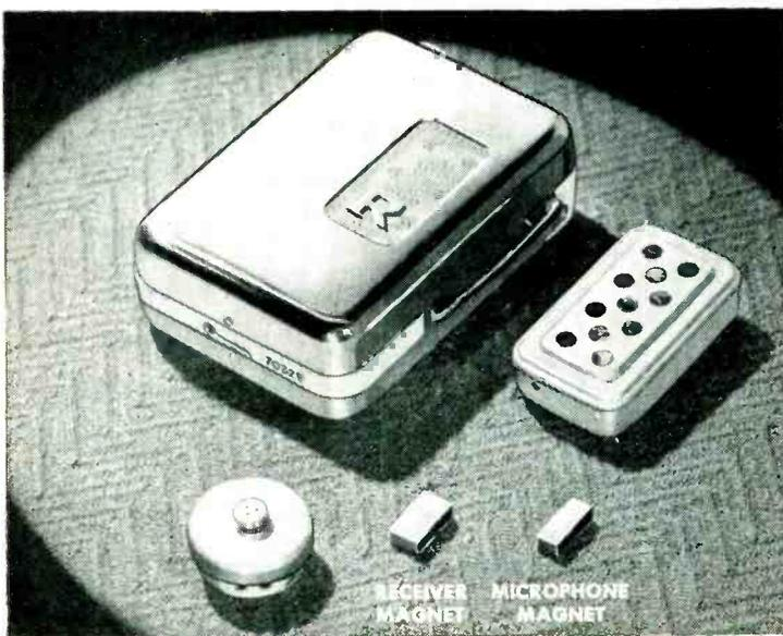
**Hearing Aids** — New all-magnetic, all-transistor "Radio-ear" hearing aid (made by E. A. Myers & Sons, Inc., Pittsburgh) uses Carboloy permanent magnets in both microphone and receiver. These magnets have eliminated hearing aid failure caused by severe heat and humidity encountered in normal use.
