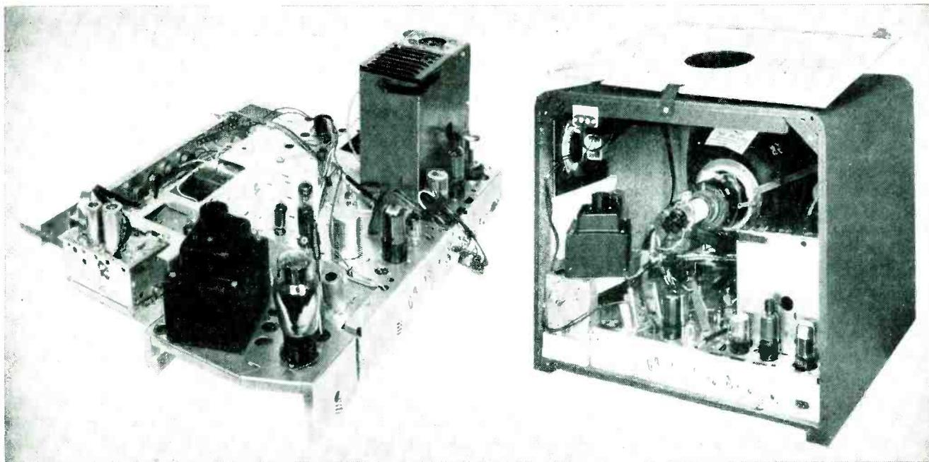
Photographs show use of subchassis to isolate power transformer and rectifier from cathode-ray tube to reduce interaction between power-frequency, scanning circuits and the electron beam. Receivers shown are 21-inch (left) and 17-inch models converted for non-synchronous operation
