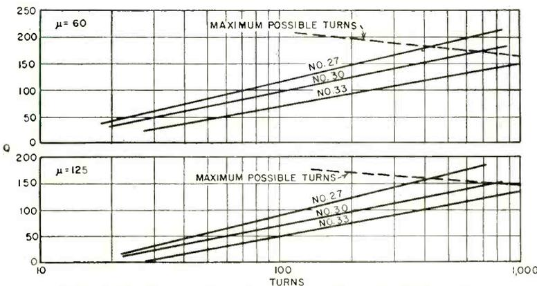
FIG. 6—Auxiliary design chart for toroids using 0.8-in. cores
