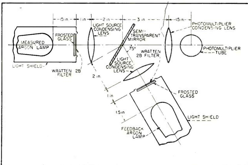
FIG. 3—Dimensions of the optical and light system employed in the photometer. Calibrated light source is introduced at left
