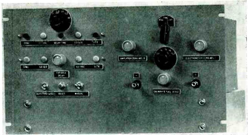
Front panel view of time-selective transient voltmeter used for cathode-ray tube persistence measurements
